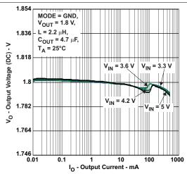
Figure 9. 1.8-V Output-Voltage Accuracy, PFM and PWM
