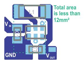
Figure 25. Recommended PCB Layout for TPS6223x-Q1
