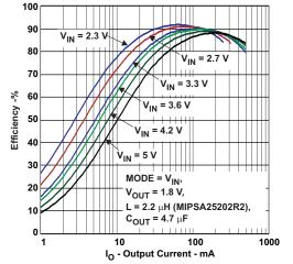
Figure 7. Efficiency: Forced PWM Mode, 1.8-V Output Voltage
