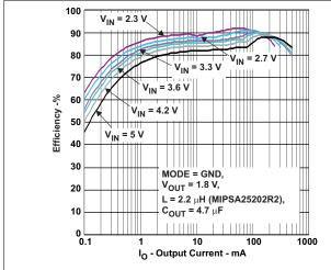
Figure 6. Efficiency: PFM and PWM Mode, 1.8-V Output Voltage
