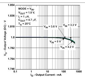
Figure 10. 1.8-V Output-Voltage Accuracy, Forced PWM Mode
