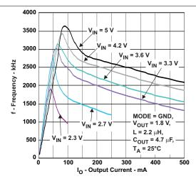
Figure 11. Switching Frequency vs Output Current, 1.8-V
