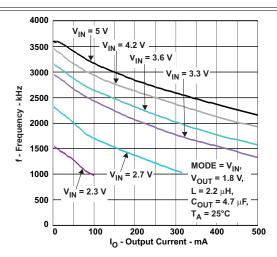
Figure 13. Switching Frequency vs Output Current, 1.8-V Output Voltage, Mode = V<sub>IN</sub>
