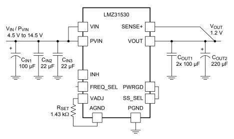
Figure 17. Typical Schematic PVIN = VIN = 4.5 V to 14.5 V, VOUT = 1.2 V
