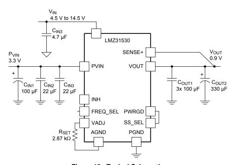
Figure 18. Typical Schematic PVIN = 3.3 V, VIN = 4.5 V to 14.5 V, VOUT = 0.9 V
