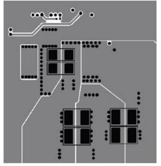
Figure 33. Typical Bottom Layer Layout
