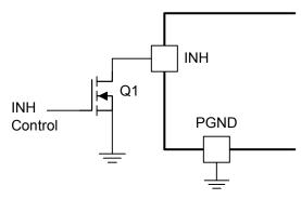
Figure 23. Typical Inhibit Control
