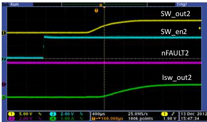
Figure 40. USB Switch2 Start-Up 1A Load
