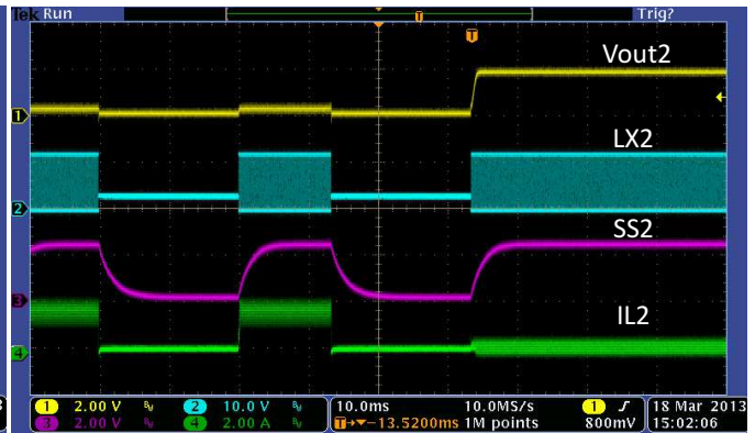
Figure 35. Hiccup Recover, Buck2=1.8V
