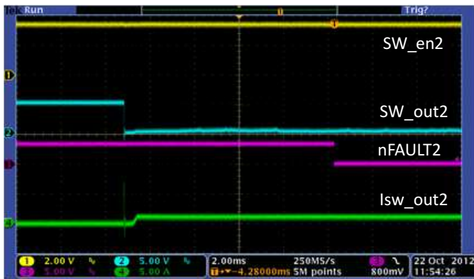
Figure 42. USB Switch2 Current Limit Operation
