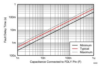
Figure 15. Adjustable Fault Delay Time
