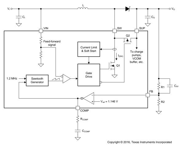
Figure 8. Boost Converter Block Diagram
