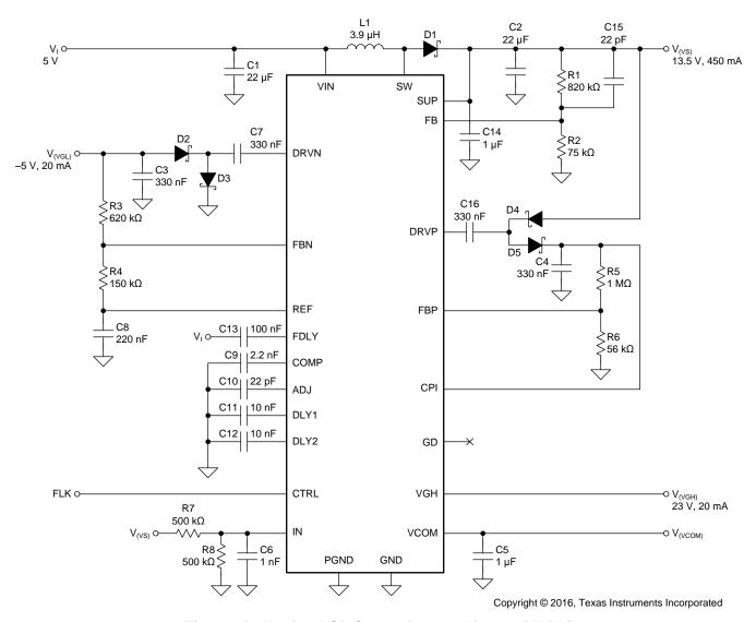
Figure 35. Monitor LCD Supply Powered from a 5-V Rail
