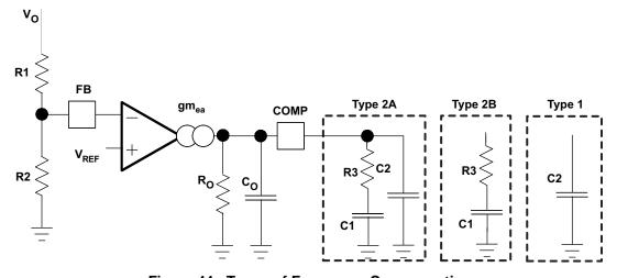
Figure 44. Types of Frequency Compensation
