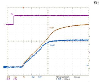
Figure 34. Ratiometric Startup With Tracking Resistors
