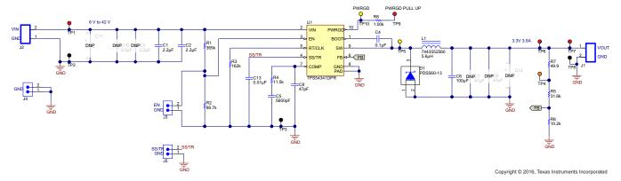
Figure 46. 3.3-V Output TPS54341 Design Example
