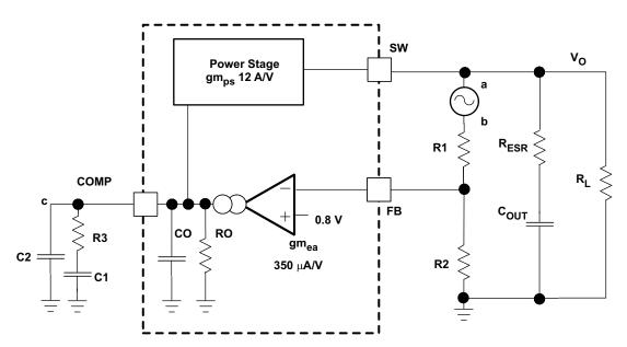
Figure 42. Small-Signal Model for Loop Response
