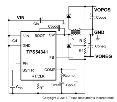
Figure 48. TPS54341 Split Rail Power Supply Based on the Application Note, SLVA369
