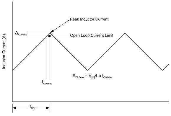
Figure 37. Current Limit Delay
