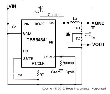
Figure 47. TPS54341 Inverting Power Supply Based on the Application Note, SLVA317
