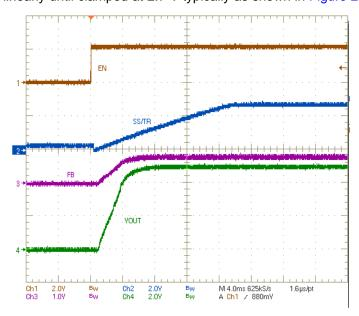
Figure 28. Operation of SS/TR Pin When Starting
