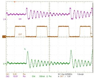
Figure 41. Plot of Synchronizing in Eco-mode
