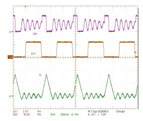
Figure 39. Plot of Synchronizing in CCM
