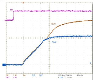
Figure 36. Simultaneous Startup With Tracking Resistor
