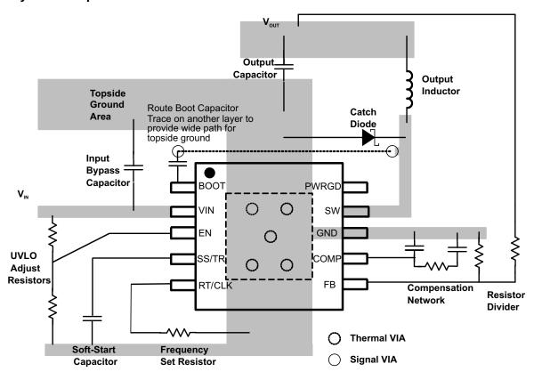
Figure 68. PCB Layout Example
