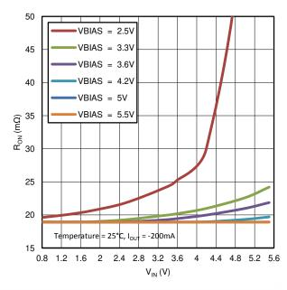
Figure 32. R<sub>ON</sub> vs. V<sub>IN</sub> (Single Channel)
