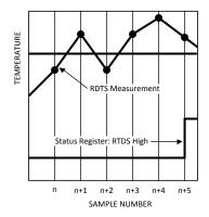
Figure 6-8. Fault Queue Temperature Response Diagram
