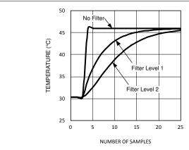
Figure 6-5. Step Response of the Digital Filter
