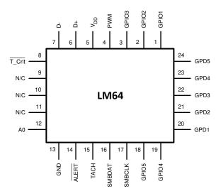
Figure 4-1. 24-pin WQFN Package
