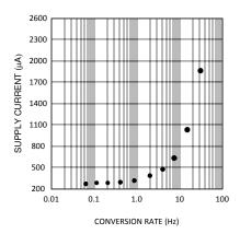
Figure 6-1. Supply Current vs Conversion Rate
