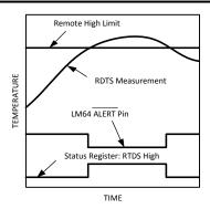
Figure 6-2. ALERT Output as Temperature Comparator Response Diagram
