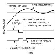
Figure 6-3. ALERT Output as an Interrupt Temperature Response Diagram
