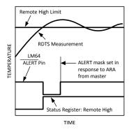
Figure 6-4. ALERT Output as an SMBus ALERT Temperature Response Diagram
