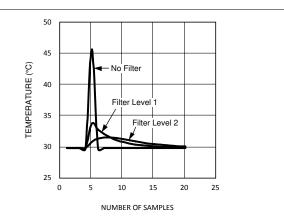
Figure 6-6. Impulse Response of the Digital Filter
