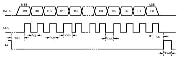
Figure 2. Serial Data Timing Diagram
