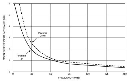
Figure 1. OSCin Input Impedance
