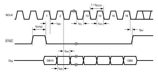
Figure 1. Serial Timing Diagram
