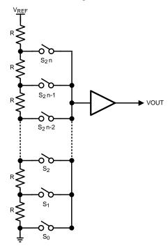
Figure 27. DAC Resistor String
