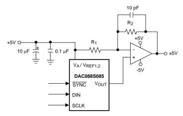
Figure 32. Bipolar Operation
