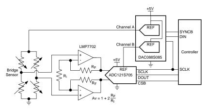
Figure 39. Driving an ADC Reference
