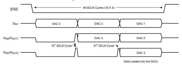
Figure 31. Daisy Chain Timing Diagram
