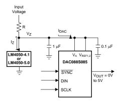
Figure 44. The LM4050 as a Power Supply
