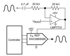
Figure 41. Programmable Attenuator Diagram
