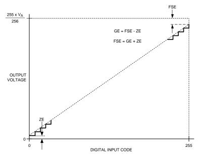
Figure 40. I/O Transfer Characteristic
