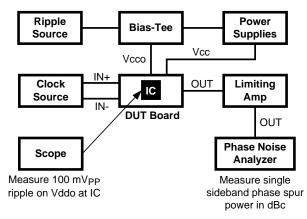
Figure 13. PSRR Test Setup
