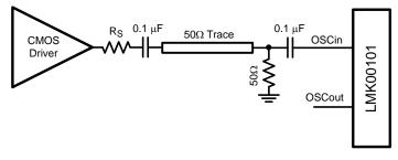
Figure 11. Driving OSCin with a Single-Ended External Clock
