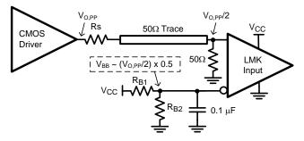
Figure 10. Single-Ended LVCMOS Input, DC Coupling with Common Mode Biasing
