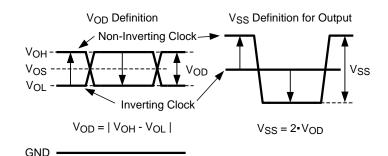
Figure 8. Two Different Definitions for Differential Output Signals
