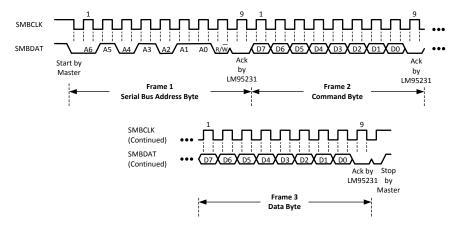
Figure 6-3. Serial Bus Write to the internal Command Register followed by a Data Byte
