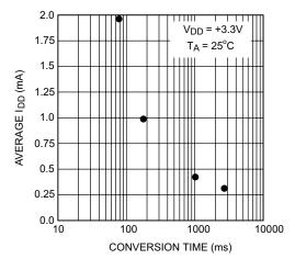
Figure 5-4. Conversion Rate Effect on Average Power Supply Current
