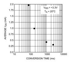
Figure 6-1. Conversion Rate Effect on Power Supply Current
