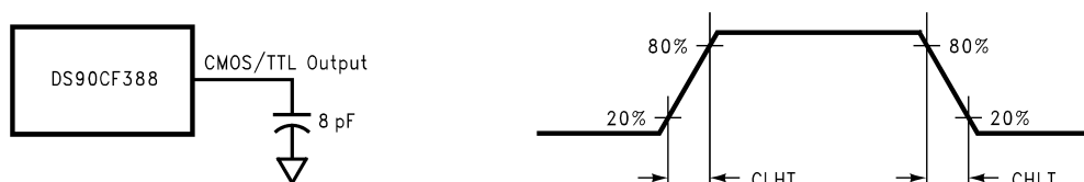
Figure 4. DS90CF388 (Receiver) CMOS/TTL Output Load and Transition Times
