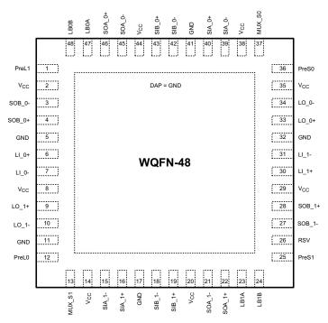
Figure 4-1. NJU Package 48-Pin WQFN Top View
