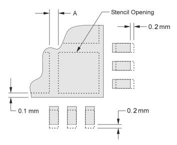
Figure 10-1. No Pullback WQFN, Single Row Reference Diagram
