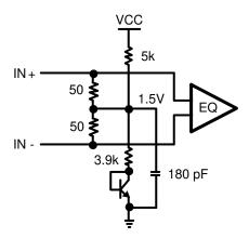
Figure 7-1. Receiver Input Termination and Bias Circuit
