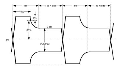
Figure 5-3. Test Condition for Output Pre-Emphasis Duration
