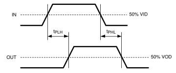
Figure 5-2. Propagation Delay From Input to Output
