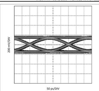
Figure 8-9. Eye Measured at Point (D), Pre-Emph = -9 dB
