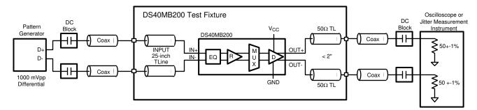
Figure 6-1. AC Test Circuit
