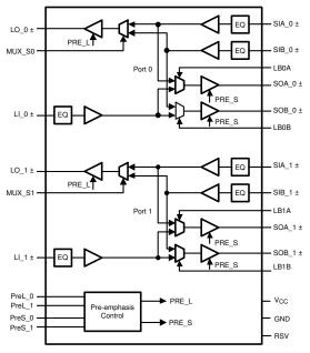
All CML inputs and outputs must be AC coupled for optimal performance.
