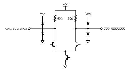
Figure 3. Equivalent SDO Output Circuit (SDO, SDO, SCO/SDO2, SCO/SDO2)
