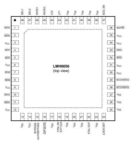
The exposed die attach pad is the primary negative electrical terminal for this device. It must be connected to the negative power supply voltage.
