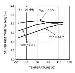
Figure 16. Driver Rise Time as a Function of Temperature
