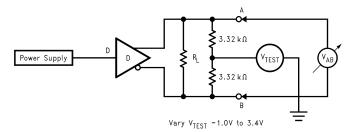
Figure 4. Differential Driver Full Load Test Circuit
