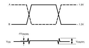
Figure 3. Differential Driver Waveforms
