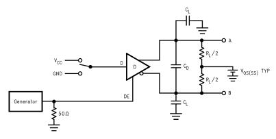
Figure 9. Driver TRI-STATE Delay Test Circuit
