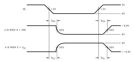
Figure 10. Driver TRI-STATE Delay Waveforms
