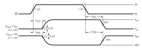
Figure 15. Receiver TRI-STATE Delay Waveforms
