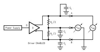
Figure 2. Differential Driver Test Circuit
