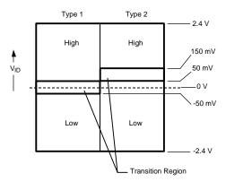
Figure 1. M-LVDS Receiver Input Thresholds
