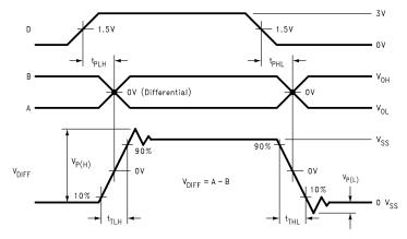
Figure 8. Driver Propagation Delays and Transition Time Waveforms
