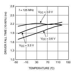
Figure 17. Driver Fall Time as a Function of Temperature
