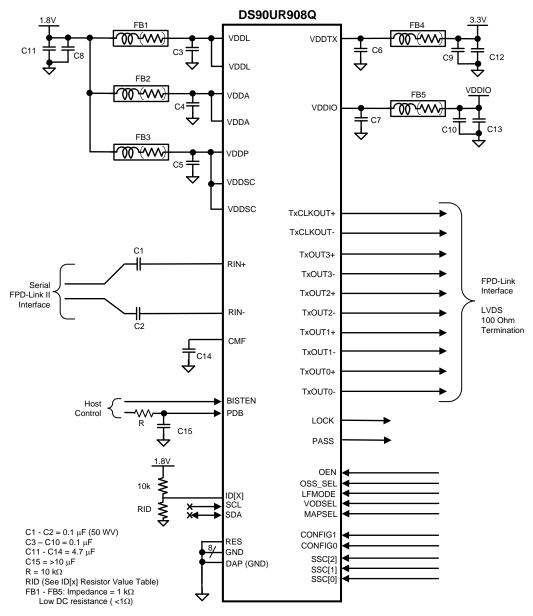
Figure 25. DS90UR908Q Typical Connection Diagram
