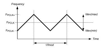
Figure 17. SSCG Waveform
