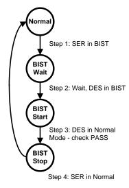
Figure 19. BIST Mode Flow Diagram
