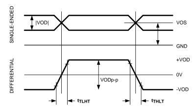
Figure 8. FPD-Link (LVDS) Single-ended and Differential Waveforms
