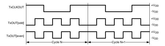
Figure 2. Checkerboard Data Pattern
