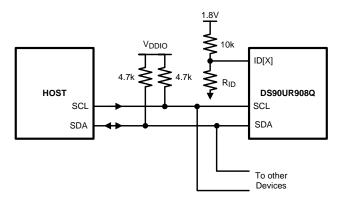
Figure 21. Serial Control Bus Connection
