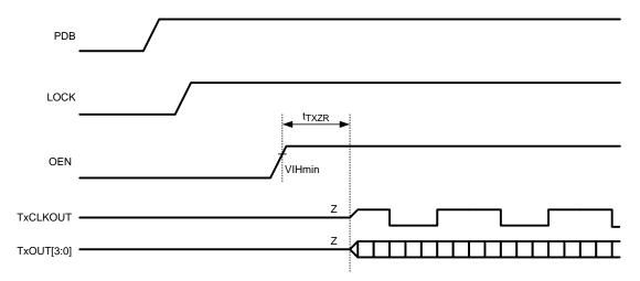
Figure 6. FPD-Link Outputs Enable Delay
