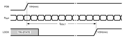
Figure 7. PLL Lock Times
