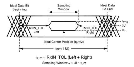
Figure 10. Receiver Input Jitter Tolerance
