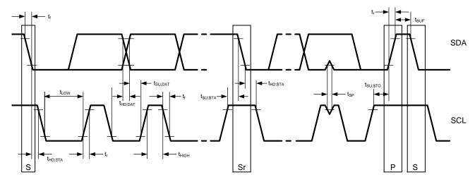
Figure 12. Serial Control Bus Timing Diagram
