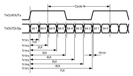
Figure 9. FPD-Link Transmitter Pulse Positions
