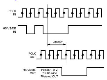
Figure 14. Video Control Signal Filter Wavefrom
