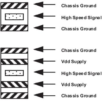
Figure 8-4. Alternative PCB Stripline Layer Stacking
