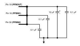
Figure 6-4. Power Feedback Connection
