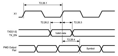
Figure 4-24. RMII Transmit Timing
