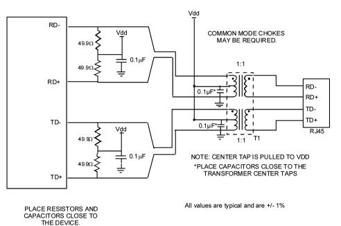
Figure 6-2. 10/100-Mb/s Twisted-Pair Interface
