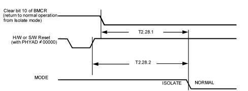
Figure 4-26. Isolation Timing
