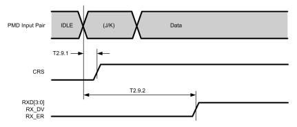
Figure 4-9. 100BASE-TX Receive Packet Latency Timing
