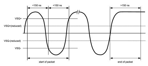
Figure 5-9. 10BASE-T Twisted-Pair Smart Squelch Operation
