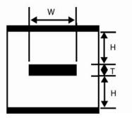
W = Width of the trace H = Height of dielectric above the return plane T = Trace thickness Er = Relative permittivity of the dielectric
