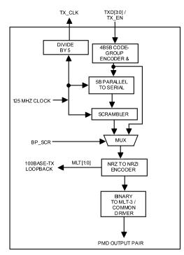
Figure 5-5. 100BASE-TX Transmit Block Diagram
