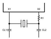
Figure 6-3. Crystal Oscillator Circuit
