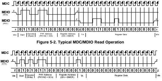
Figure 5-3. Typical MDC/MDIO Write Operation
