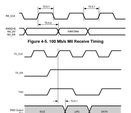
Figure 4-6. 100BASE-TX MII Transmit Packet Latency Timing
