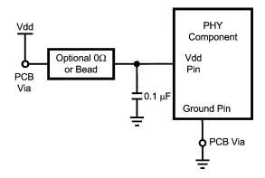
Figure 7-1. Vdd Bypass Layout
