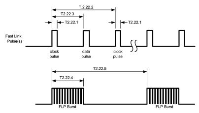
Figure 4-20. Auto-Negotiation Fast Link Pulse (FLP) Timing
