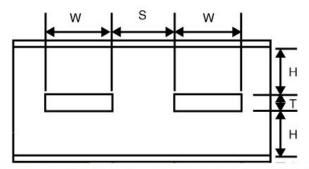
W = Width of the trace H = Height of dielectric above the return plane T = Trace thickness S = space between traces Er = Relative permittivity of the dielectric
