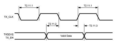
Figure 4-11. 10-Mb/s MII Transmit Timing
