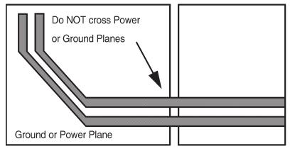
Figure 8-2. Differential Signal Pair-Plane Crossing
