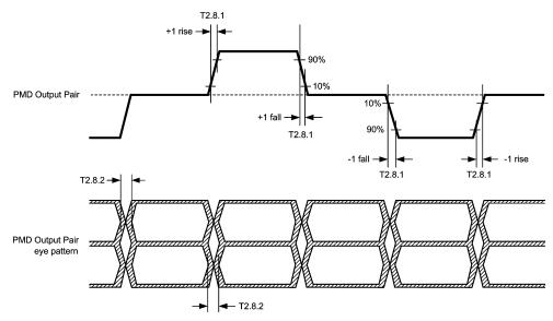
Figure 4-8. 100BASE-TX Transmit Timing (t<sub>R/F</sub> and Jitter)
