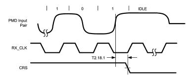
Figure 4-16. 10BASE-T Receive Timing (End of Packet)
