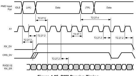
Figure 4-25. RMII Receive Timing
