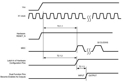
Figure 4-1. Power Up Timing
