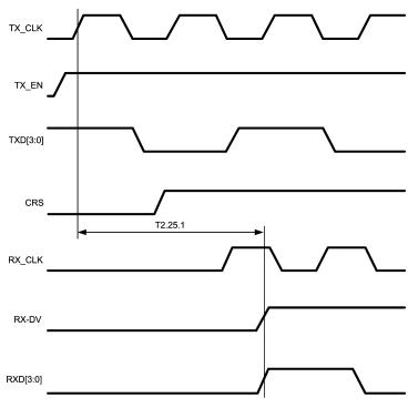
Figure 4-23. 10-Mb/s Internal Loopback Timing
