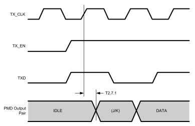
Figure 4-7. 100BASE-TX Transmit Packet Deassertion Timing
