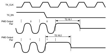
Figure 4-14. 10BASE-T Transmit Timing (End of Packet)
