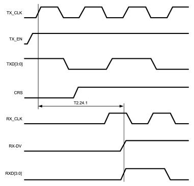
Figure 4-22. 100-Mb/s Internal Loopback Timing
