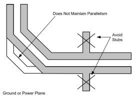
Figure 8-1. Differential Signal Pair – Stubs
