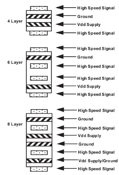
Figure 8-3. PCB Stripline Layer Stacking
