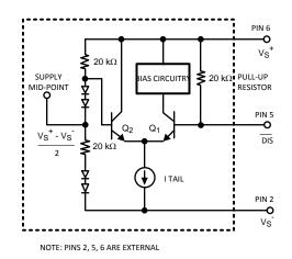
Figure 22. DIS Pin Simplified Schematic
