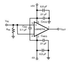
Figure 20. Alternate Unity Gain Configuration
