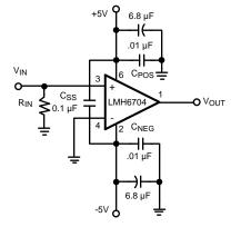
Figure 17. Recommended Gain of +2 Circuit
