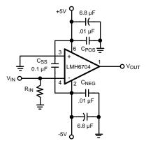
Figure 19. Recommended Gain of -1 Circuit
