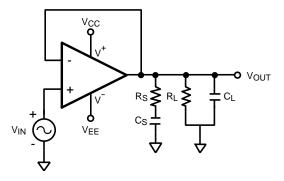
Figure 47. Snubber Network to Improve Phase Margin
