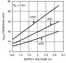
Figure 22. Negative Output Swing vs Supply Voltage
