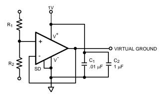
Figure 54. Virtual Ground Circuit
