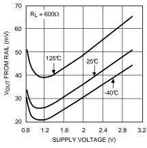
Figure 23. Positive Output Swing vs Supply Voltage
