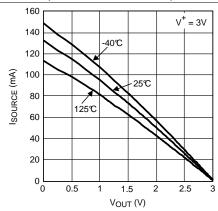
Figure 19. Sourcing Current vs Output Voltage
