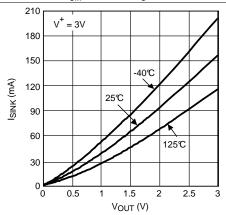
Figure 20. Sinking Current vs Output Voltage
