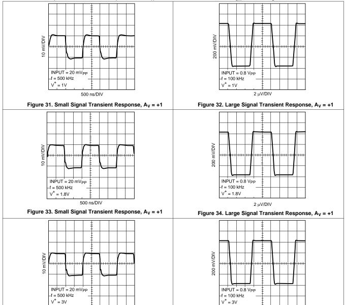
Figure 35. Small Signal Transient Response,  $A_V = +1$ Figure 36. Large Signal Transient Response,  $A_V = +1$
