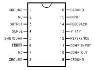
Note: Pins 1, 8, 9, 16 must be shorted together on customer PC board application
