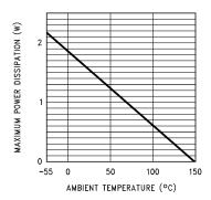
Figure 30. Power Derating Curve for LP2953
