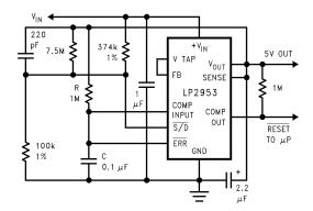
Figure 41. 5V Regulator with Timed Power-On Reset, Snap-On/Snap-Off Feature and Hysteresis
