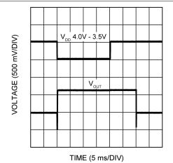
Figure 12. Charge Pump Automatic Gain Change (LED  $V_F = 3.6 \text{ V}$ )
