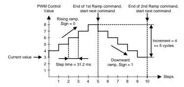
Figure 25. Example of 2 Sequential Ramp Commands.
