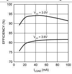
Figure 6. Charge Pump Efficiency vs Load Current
