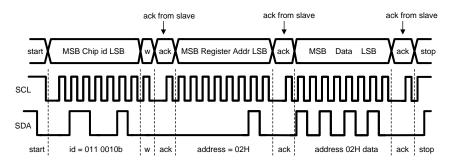
Figure 23. Register Write Format
