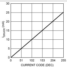
Figure 4. LED Current vs Current Register Code
