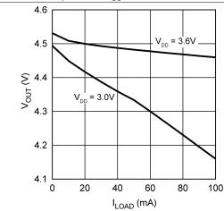
Figure 8. Charge Pump Output Voltage vs Load Current
