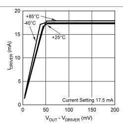
Figure 3. LED Current vs Output Pin Headroom Voltage
