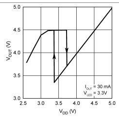
Figure 10. Charge Pump Automatic Gain Change Hysteresis
