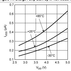
Figure 13. Standby Current vs Input Voltage
