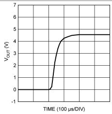
Figure 11. Charge Pump Start-Up in 1.5× Mode: No Load
