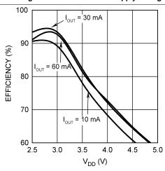
Figure 7. Charge Pump Efficiency vs Input Voltage 1.5x Mode
