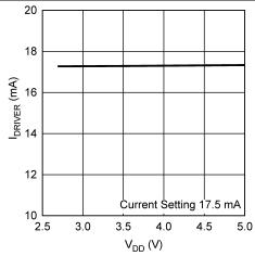
Figure 5. LED Current vs Supply Voltage
