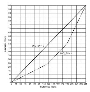
Figure 16. Logarithmic and Linear PWM Adjustment Curves
