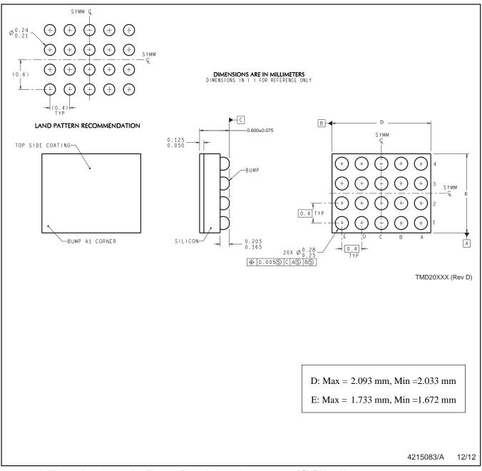
NOTES: A. All linear dimensions are in millimeters. Dimensioning and tolerancing per ASME Y14.5M-1994. B. This drawing is subject to change without notice.
