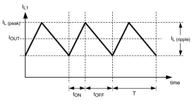
Figure 23. Relationship Between I<sub>OUT</sub>, I<sub>L(peak)</sub> and I<sub>L(ripple)</sub>
