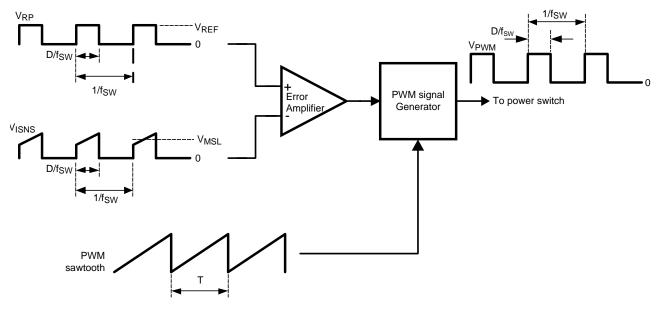
Figure 21. Implementation of the PWM Switching Signal
