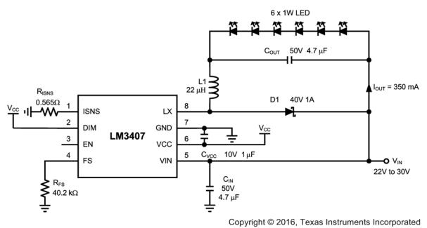
Figure 26. LM3407 6 LED Example Schematic
