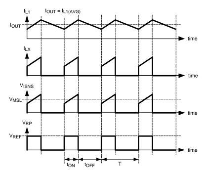
Figure 19. LM3407 Switching Waveforms
