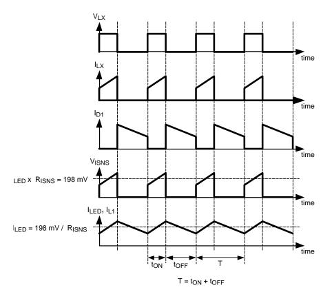
Figure 18. Operating Waveforms of a Floating Buck Converter
