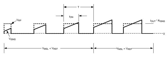
Figure 22. Waveforms of V<sub>ISNS</sub> and V<sub>RP</sub> Under Closed-Loop Operation
