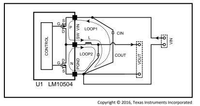
Figure 31. Schematic of LM10504 Highlighting Layout Sensitive Nodes
