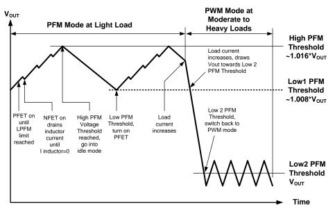
Figure 20. PFM vs PWM Operation
