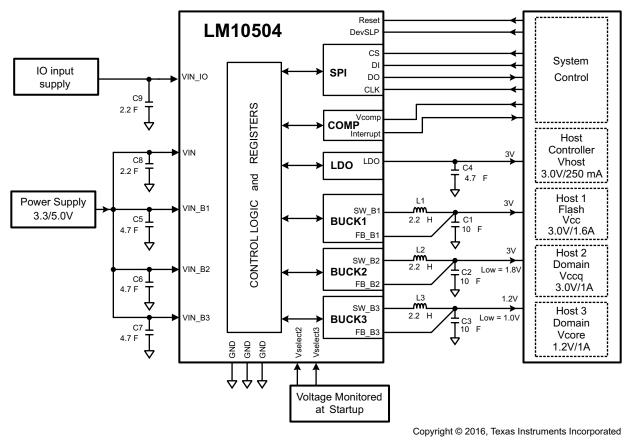
Figure 25. Typical Application Diagram
