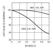
Figure 26. Typical Variation in Capacitance vs DC Bias
