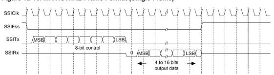
Figure 12-10. MICROWIRE Frame Format (Single Frame)
