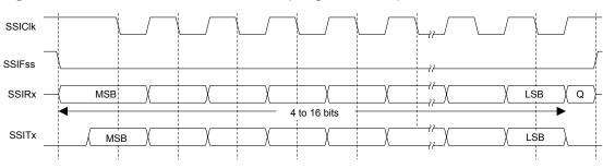
Figure 12-7. Freescale SPI Frame Format (Single Transfer) with SPO=1 and SPH=0
