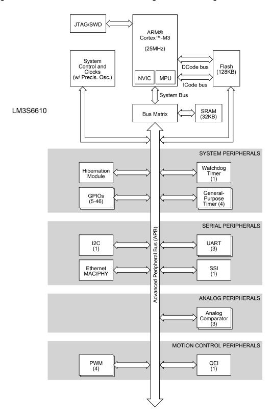
Figure 1-1. Stellaris LM3S6610 Microcontroller High-Level Block Diagram
