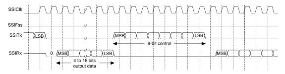
Figure 12-11. MICROWIRE Frame Format (Continuous Transfer)
