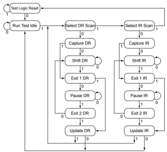
Figure 4-2. Test Access Port State Machine
