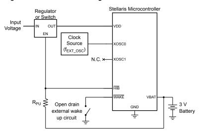
Figure 6-3. Clock Source Using Dedicated Oscillator
