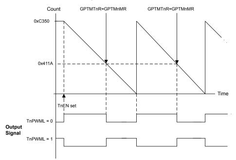
Figure 9-4. 16-Bit PWM Mode Example
