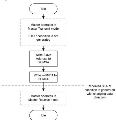
Figure 13-11. Master Burst RECEIVE after Burst SEND
