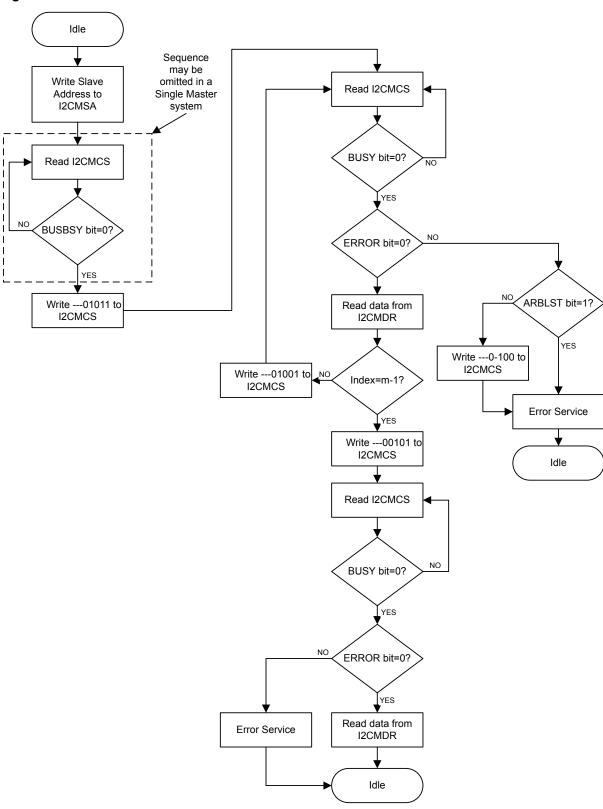
Figure 13-10. Master Burst RECEIVE
