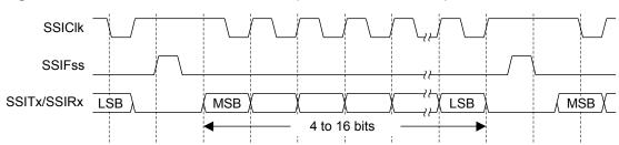
Figure 12-8. Freescale SPI Frame Format (Continuous Transfer) with SPO=1 and SPH=0
