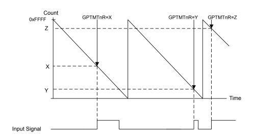
Figure 9-3. 16-Bit Input Edge Time Mode Example
