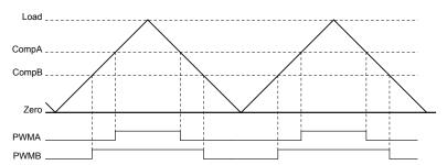
Figure 16-5. PWM Generation Example In Count-Up/Down Mode
