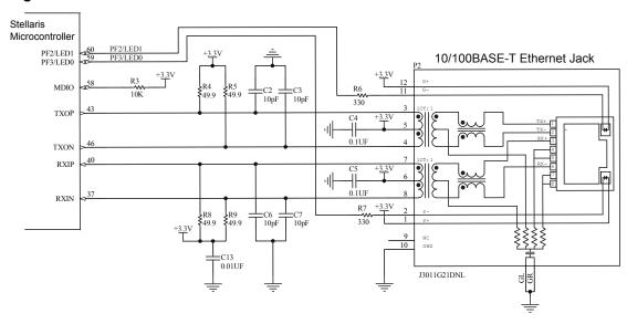
Figure 14-4. Interface to an Ethernet Jack
