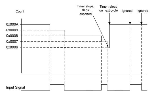
Figure 9-2. 16-Bit Input Edge Count Mode Example
