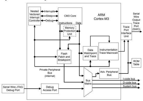
Figure 2-1. CPU Block Diagram
