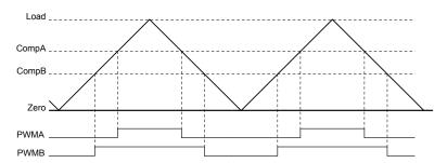
Figure 14-5. PWM Generation Example In Count-Up/Down Mode
