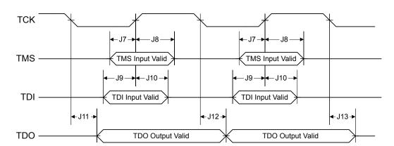
Figure 18-3. JTAG Test Access Port (TAP) Timing
