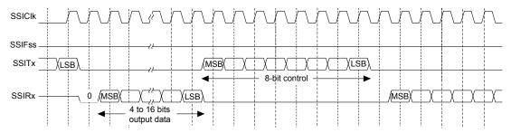
Figure 12-11. MICROWIRE Frame Format (Continuous Transfer)
