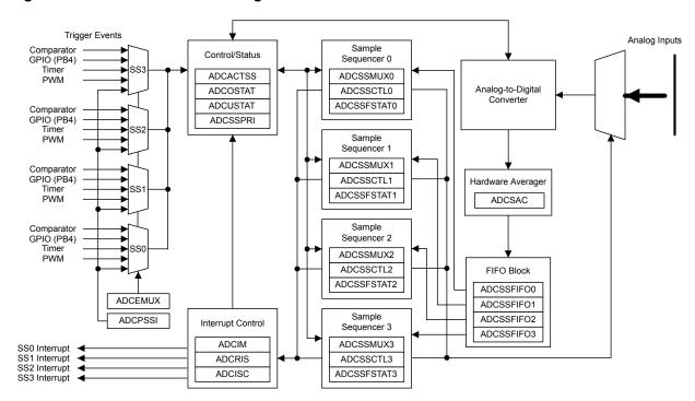
Figure 10-1. ADC Module Block Diagram
