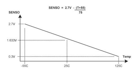
Figure 10-5. Internal Temperature Sensor Characteristic
