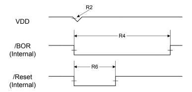
Figure 18-8. Software Reset Timing
