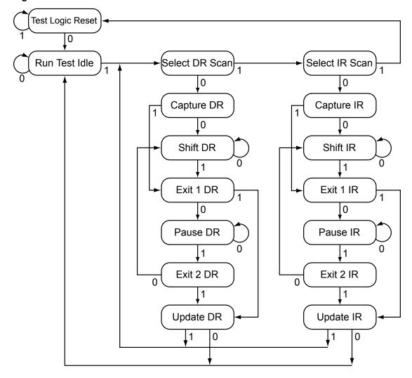
Figure 4-2. Test Access Port State Machine
