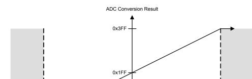
Figure 10-2. Differential Sampling Range,  $V_{IN\_ODD}$  = 1.5 V
