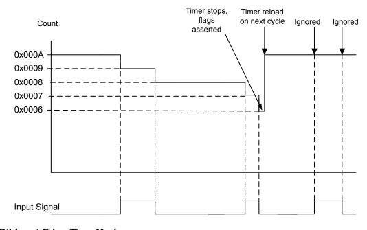
Figure 8-2. 16-Bit Input Edge Count Mode Example
