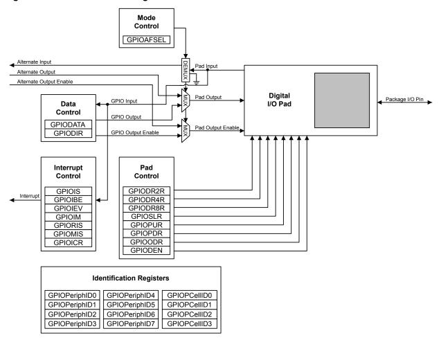
Figure 7-2. GPIO Port Block Diagram
