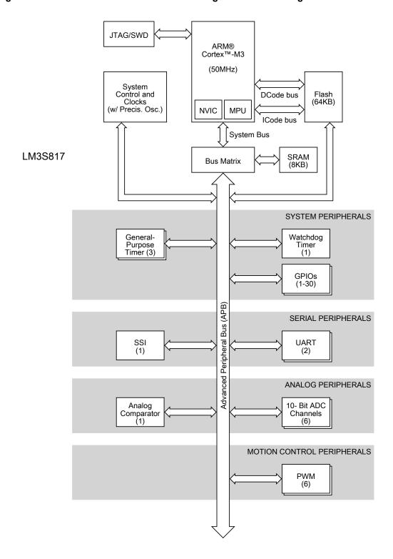
Figure 1-1. Stellaris LM3S817 Microcontroller High-Level Block Diagram
