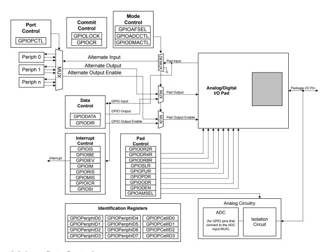
Figure 9-2. Analog/Digital I/O Pads
