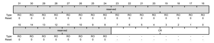
RO 0x0000.00 31.8 Software should not rely on the value of a reserved bit. To provide reserved compatibility with future products, the value of a reserved bit should be preserved across a read-modify-write operation.
