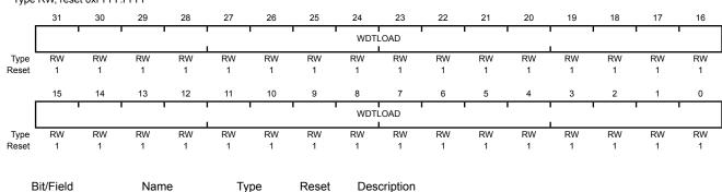
Description Type Reset 31:0 **WDTLOAD** RW 0xFFFF.FFFF Watchdog Load Value
