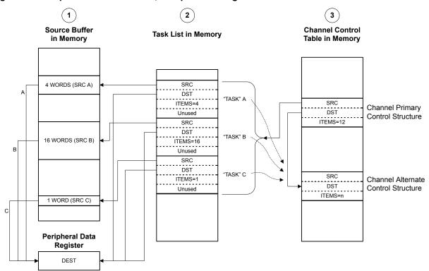
Figure 8-5. Peripheral Scatter-Gather, Setup and Configuration
