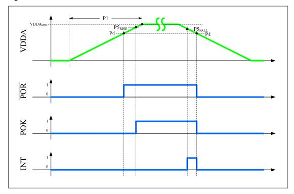
Figure 21-4. Power Assertions versus VDDA Levels
