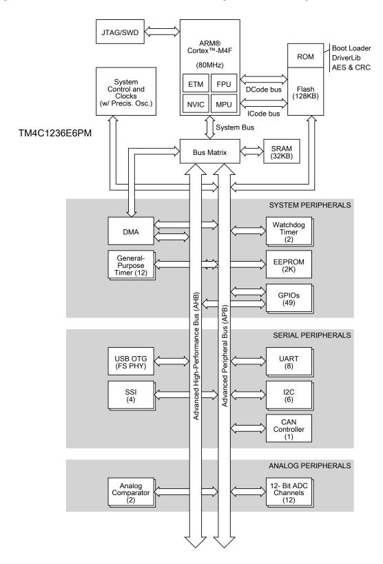
Figure 1-1. Tiva<sup>™</sup> TM4C1236E6PM Microcontroller High-Level Block Diagram
