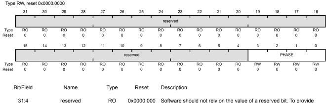
Software should not rely on the value of a reserved bit. To provide compatibility with future products, the value of a reserved bit should be preserved across a read-modify-write operation.
