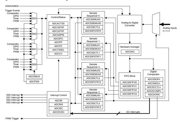
Figure 12-2. ADC Module Block Diagram
