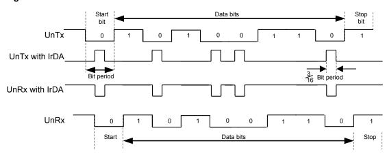
Figure 13-3. IrDA Data Modulation
