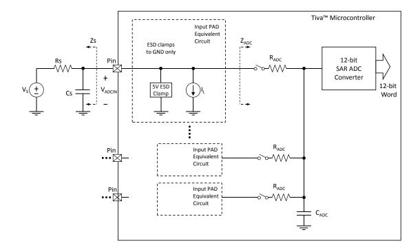
The ADC operates from both the 3.3-V analog and 1.2-V digital power supplies. The ADC clock can be configured to reduce power consumption when ADC conversions are not required (see "System Control" on page 217). The analog inputs are connected to the ADC through specially balanced input paths to minimize the distortion and cross-talk on the inputs. Detailed information on the ADC power supplies and analog inputs can be found in "Analog-to-Digital Converter (ADC)" on page 1214.
