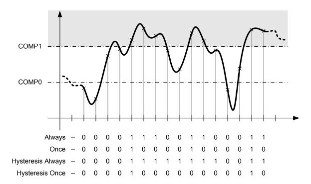
Figure 12-14. High-Band Operation (CIC=0x3)
