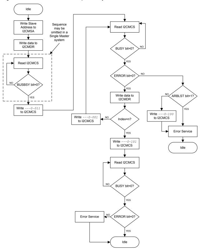
Figure 16-10. Master TRANSMIT of Multiple Data Bytes
