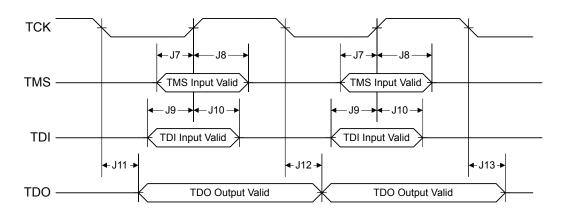
Figure 22-3. JTAG Test Access Port (TAP) Timing
