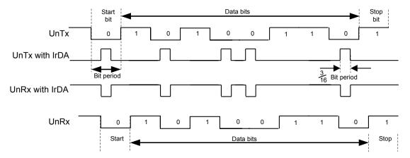
Figure 14-3. IrDA Data Modulation
