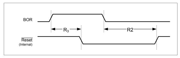
Figure 22-11. External Reset Timing (RST)
