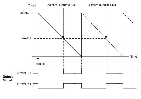
Figure 11-5. 16-Bit PWM Mode Example
