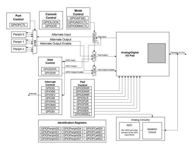
Figure 10-2. Analog/Digital I/O Pads
