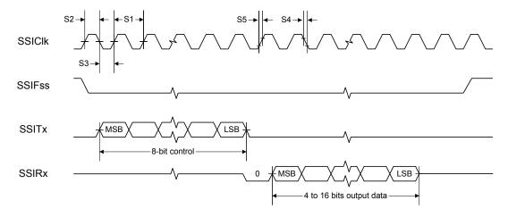
Figure 22-22. Master Mode SSI Timing for SPI Frame Format (FRF=00), with SPH=1
