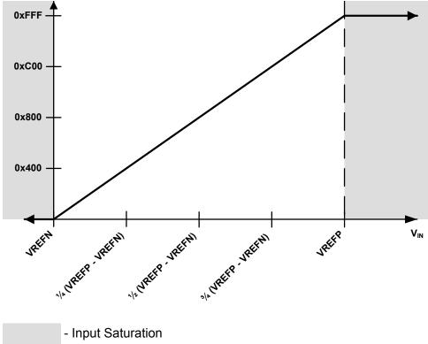
Figure 13-9. ADC Conversion Result
