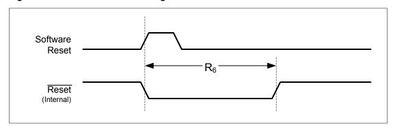
Figure 22-13. Watchdog Reset Timing
