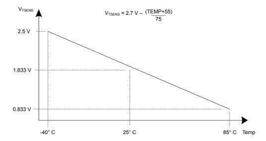
Figure 13-11. Internal Temperature Sensor Characteristic
