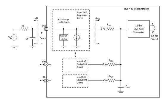
Figure 22-19. ADC Input Equivalency Diagram
