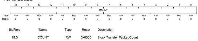
Sets the number of packets of the size defined by the  ${\tt MAXLOAD}$  bit field that are to be transferred in a block transfer.
