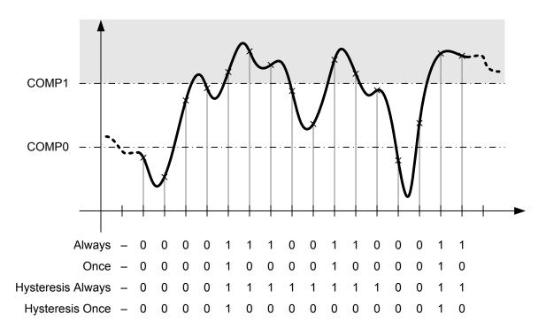
Figure 13-14. High-Band Operation (CIC=0x3)
