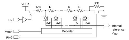
**Note:** In the figure above, N\*R represents a multiple of the R value that produces the results specified in Table 19-2 on page 1209.
