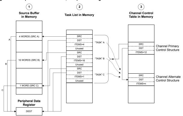
Figure 9-5. Peripheral Scatter-Gather, Setup and Configuration
