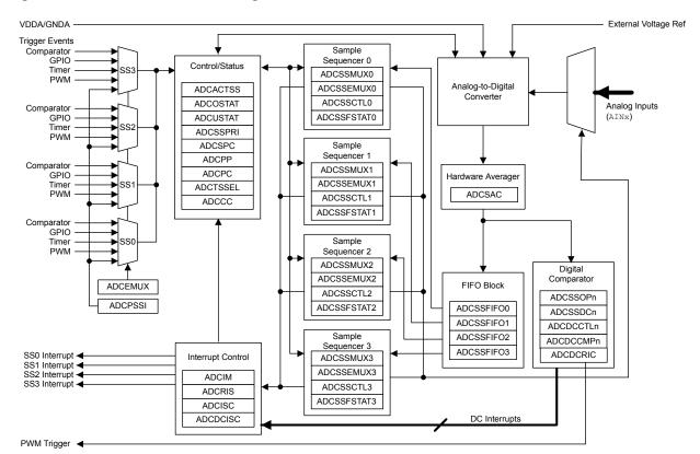
Figure 13-2. ADC Module Block Diagram
