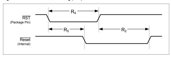
Figure 22-12. Software Reset Timing
