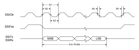
Figure 22-21. SSI Timing for MICROWIRE Frame Format (FRF=10), Single Transfer
