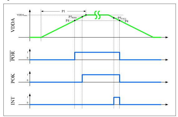
Figure 22-4. Power Assertions versus VDDA Levels
