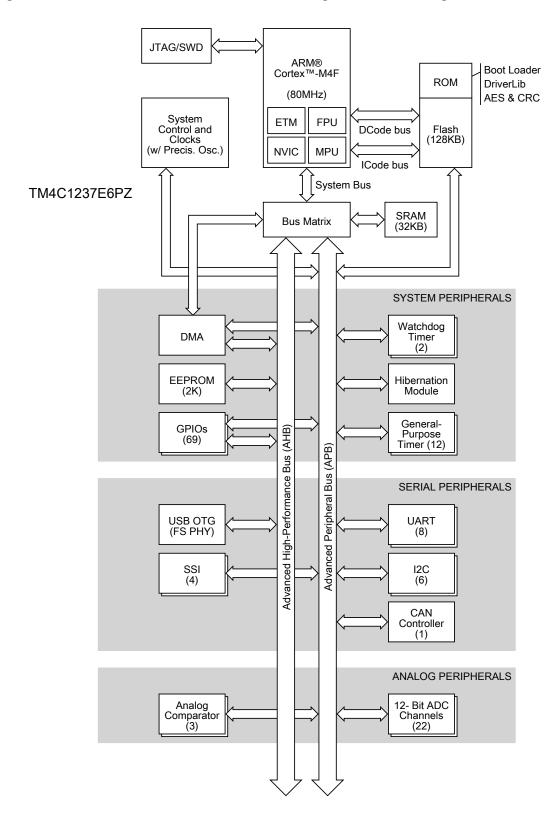
Figure 1-1. Tiva<sup>™</sup> TM4C1237E6PZ Microcontroller High-Level Block Diagram
