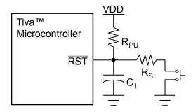
Typical  $R_{PU} = 10 \text{ k}\Omega$
