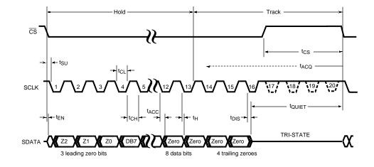
Figure 2. ADC081S101-MIL Serial Timing Diagram
