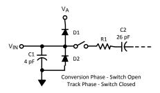
Figure 22. Equivalent Input Circuit
