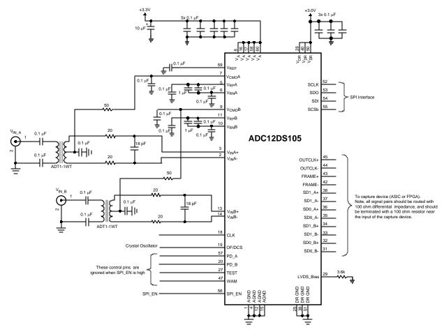
Figure 23. Application Circuit
