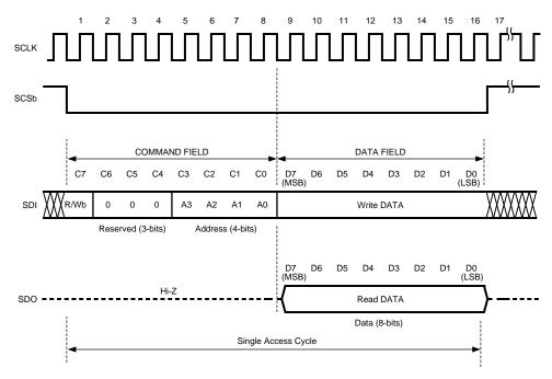
Figure 24. Serial Interface Protocol
