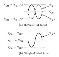
Figure 19. Expected Input Signal Range
