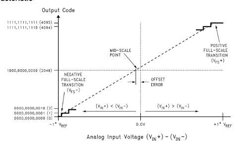
Figure 6. Transfer Characteristic
