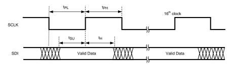
Figure 26. Write Timing
