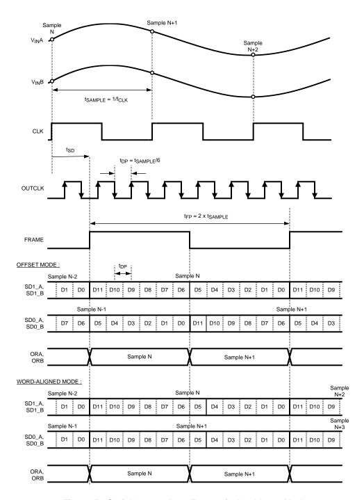
Figure 5. Serial Output Data Format in Dual-Lane Mode
