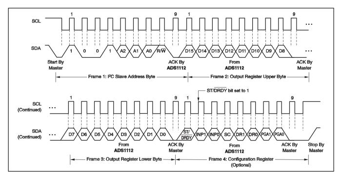
Figure 2. Timing Diagram for Reading From the ADS1112
