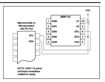
Figure 7. Using GPIO with a Single ADS1112
