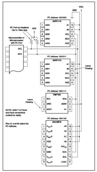
Figure 6. Connecting Multiple Device Types
