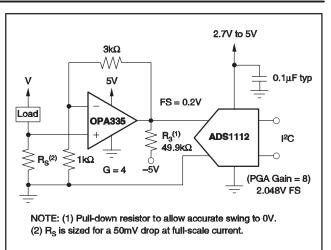
Figure 9. Low-Side Current Measurement
