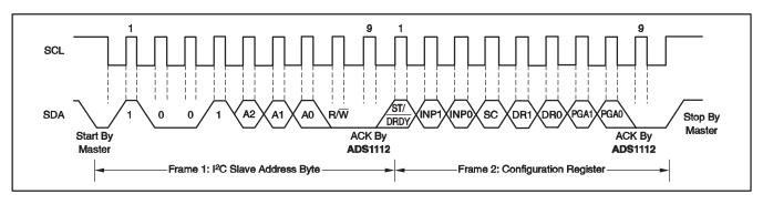
Figure 3. Timing Diagram for Writing To the ADS1112
