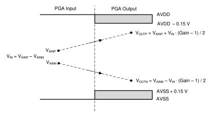
Figure 44. PGA Input/Output Range
