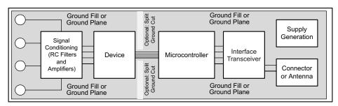
Figure 103. System Component Placement
