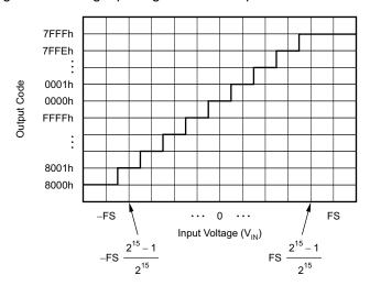
Figure 72. Code Transition Diagram
