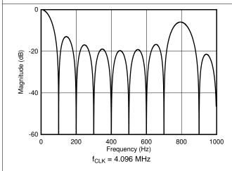
Figure 55. Digital Filter Frequency Response, Data Rate = 100 SPS
