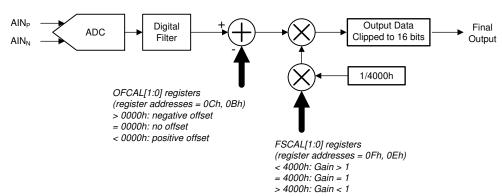
Figure 66. ADC Calibration Block Diagram
