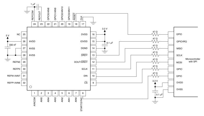
Figure 94. Serial Interface Connections
