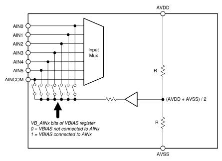
Figure 64. VBIAS Block Diagram
