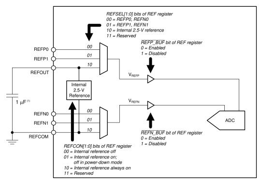
(1) The internal reference requires a minimum 1-µF capacitor connected from REFOUT to REFCOM.
