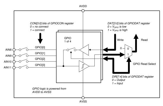
Figure 65. GPIO Block Diagram
