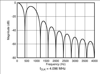
Figure 57. Digital Filter Frequency Response,
