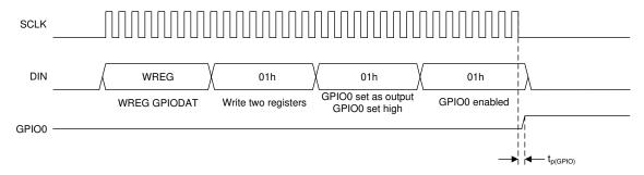
Figure 6. GPIO Switching Characteristics
