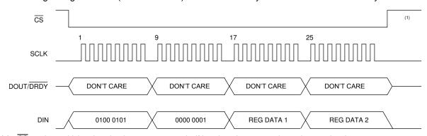
(1)  $\overline{\text{CS}}$  can be set high or kept low between commands. If kept low, the command must be completed.
