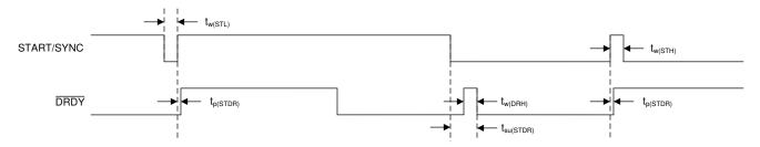
Figure 4. START/SYNC Pin Timing Requirements
