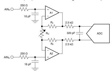
Figure 43. Simplified PGA Diagram
