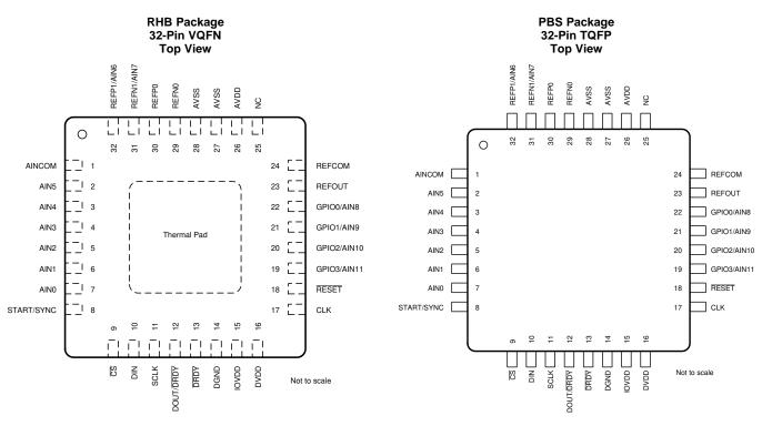
NOTE: The analog input functions (AIN6-AIN11) are not available on pins 19 to 22, 31, and 32 for the ADS114S06B.
