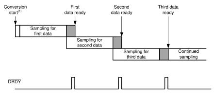
Conversions start at the rising edge of the START/SYNC pin or on the seventh SCLK falling edge for a START command.
