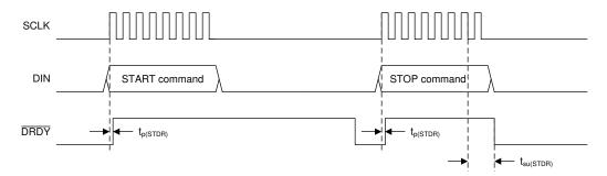
Figure 5. START Command Timing Requirements
