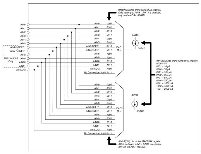
Figure 63. IDAC Block Diagram
