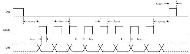
NOTE: Single-byte communication is shown. Actual communication can be multiple bytes.
