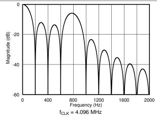
Figure 56. Digital Filter Frequency Response,
