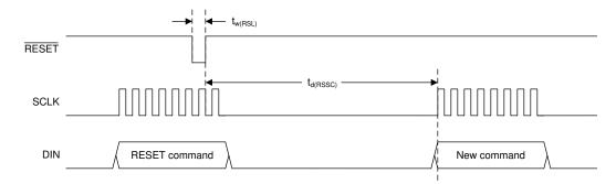
Figure 3. RESET Pin and RESET Command Timing Requirements
