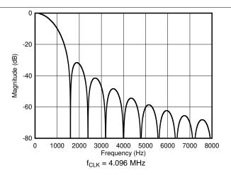
Figure 58. Digital Filter Frequency Response,
