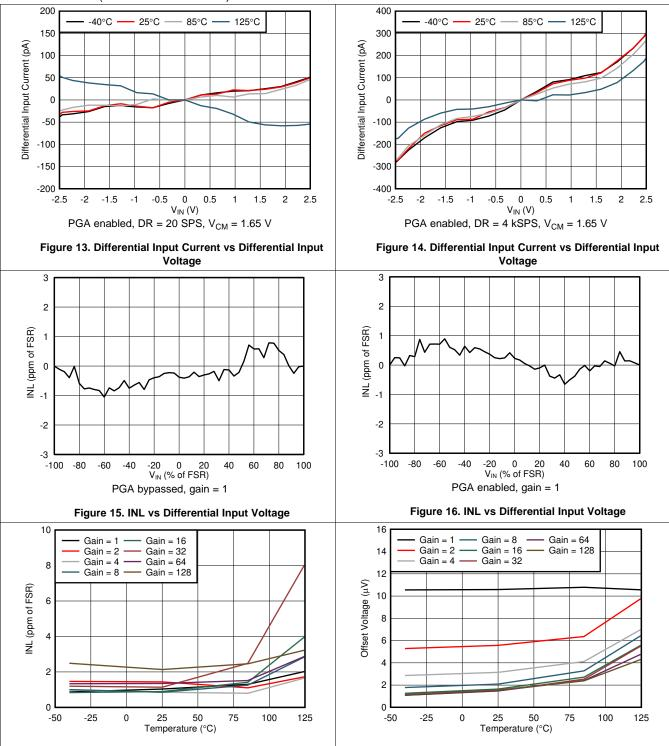
Figure 17. INL vs Temperature
