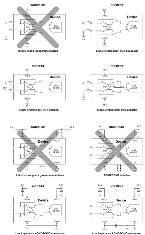
Figure 100. Do's and Don'ts Circuit Connections
