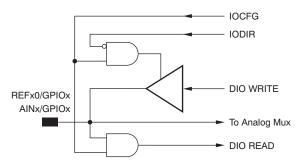
Figure 69. Analog and Data Interface Pin
