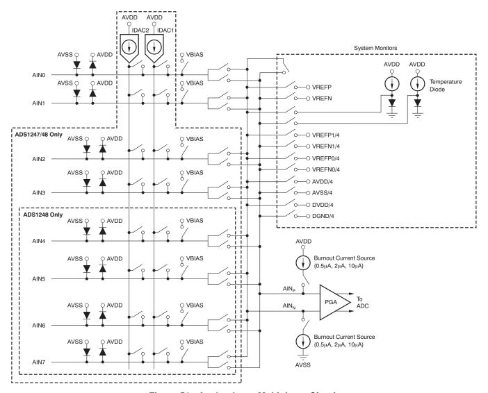
Figure 51. Analog Input Multiplexer Circuit
