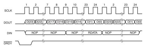
Figure 82. Using RDATA in Full-Duplex Mode
