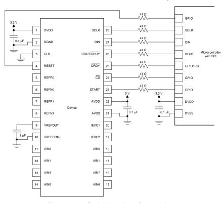
Figure 110. Serial Interface Connections
