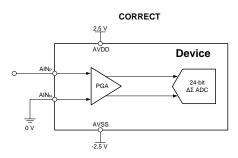
Input grounded, bipolar supply
