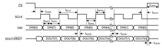
Figure 1. Serial Interface Timing, DRDY MODE Bit = 0
