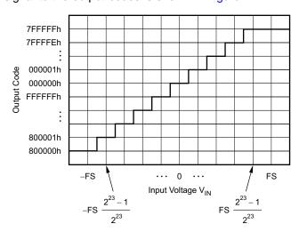
Figure 77. Code Transition Diagram
