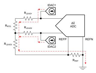
Figure 116. Example of Lead Wire Compensation
