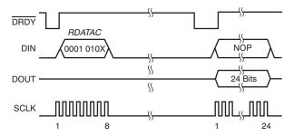
Figure 83. Read Data Continuously
