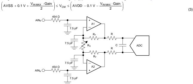
Figure 52. Simplified Diagram of the PGA
