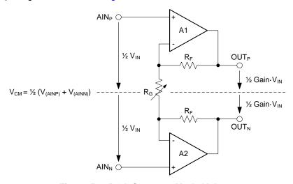
Figure 53. PGA Common-Mode Voltage
