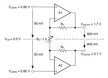
Figure 54. Example where V<sub>CM</sub> is at Lowest Limit
