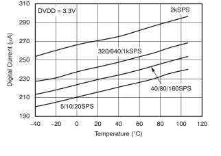
Figure 48. Digital Supply Current vs Temperature
