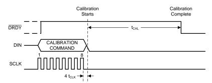
Figure 86. Calibration Command
