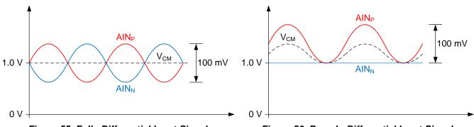
Figure 55. Fully-Differential Input Signal
