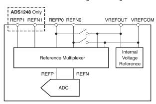
Figure 68. Reference Input Multiplexer
