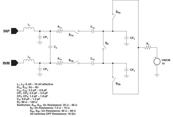
A. All Switches are ON in sampling phase which is approximately one half of a clock period.
