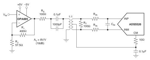
Figure 41. Converting a Single-Ended Input Signal to a Differential Signal Using an RF Transformer
