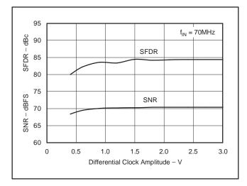
Figure 49. AC Performance vs Clock Amplitude
