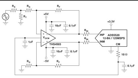
Figure 42. Using the THS4503 with the ADS5520
