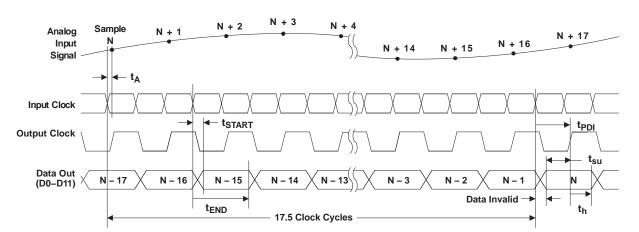
A. It is recommended that the loading at CLKOUT and all data lines are accurately matched to ensure that the above timing matches closely with the specified values.
