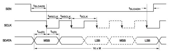
Figure 4. Serial Programming Interface Timing Diagram
