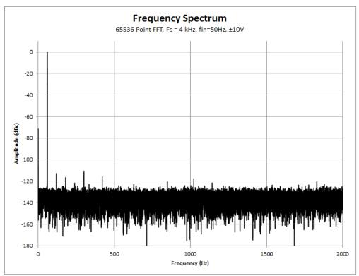
Figure 87. Frequency Spectrum for a Sinusoidal ±10-V Signal at 50 Hz
