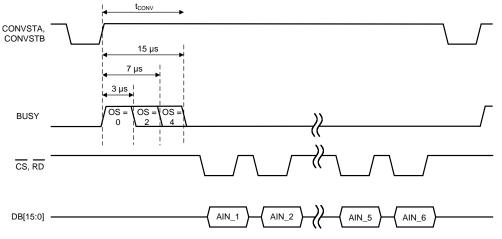
Figure 71. OSR Mode Operation Timing Diagram
