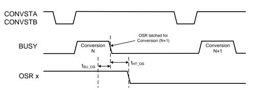
Figure 7. Oversampling Mode Timing Diagram
