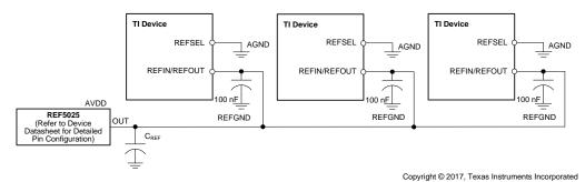
Figure 65. Multiple Devices Connected Using an External Reference
