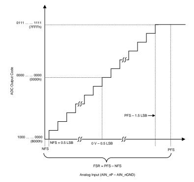
Figure 66. 16-Bit ADC Transfer Function (Twos Complement Binary Format)
