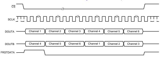
Figure 69. Data Read Back in the Serial Interface Using Either DOUTA or DOUTB Timing Diagram
