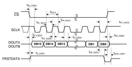
Figure 5. Serial Data Read Operation Timing Diagram
