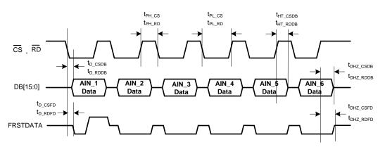
Figure 3. Parallel Data Read Operation,  $\overline{CS}$  and  $\overline{RD}$  Tied Together
