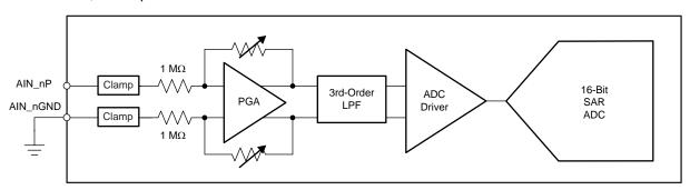
Figure 52. Front-End Circuit Schematic for Each Analog Input Channel
