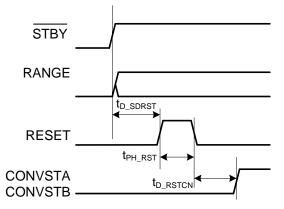
Figure 9. Exit Shutdown Mode Timing Diagram
