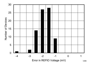
Figure 59. Solder Heat Shift Distribution Histogram
