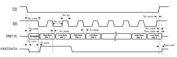
Figure 6. Byte Mode Data Read Operation Timing Diagram
