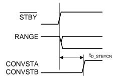
Figure 8. Exit Standby Mode Timing Diagram
