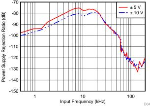
Figure 88. PSRR Across Frequency (With Decoupling Capacitor)
