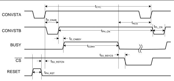
Figure 1. CONVST Control Timing Diagram
