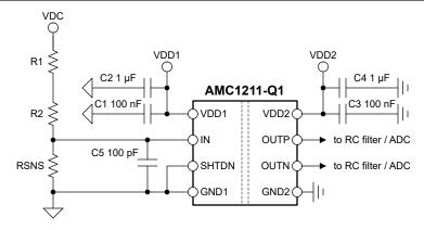
Figure 8-5. Decoupling of the AMC1211-Q1
