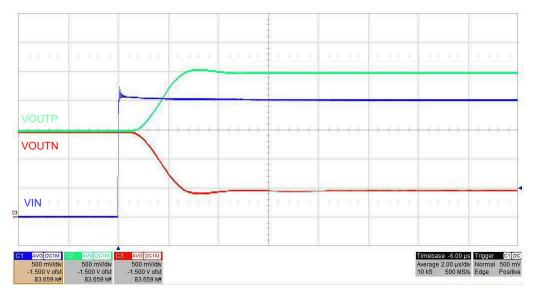
Figure 8-4. Step Response of the AMC1211-Q1
