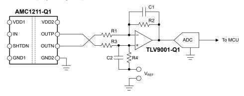
Figure 8-3. Connecting the AMC1211-Q1 Output to a Single-Ended Input ADC
