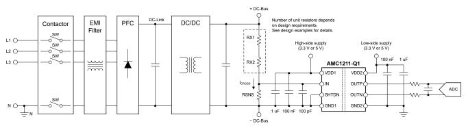
Figure 8-1. Using the AMC1211-Q1 for DC Bus Voltage Sensing in an OBC
