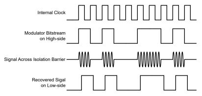
Figure 7-1. OOK-Based Modulation Scheme
