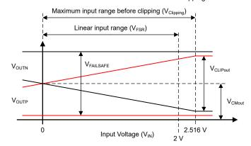
Figure 7-2. Output Behavior of the AMC1211-Q1
