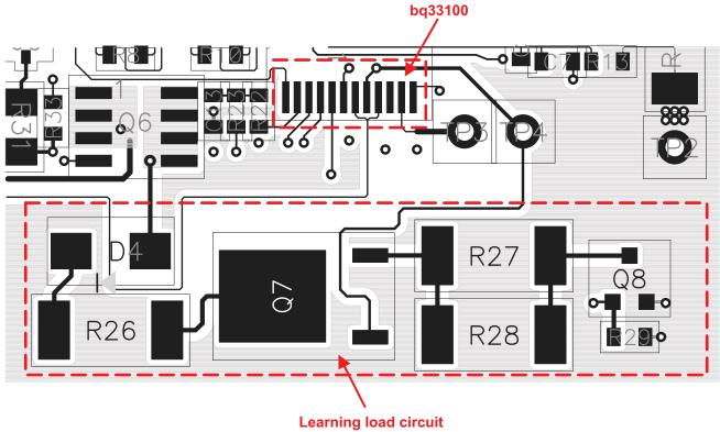
with extra copper for heat dissipation
