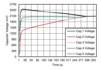
Figure 19. Voltage Convergence During Capacitor Balancing
