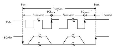
Figure 2. SMBus t<sub>TIMEOUT</sub>
