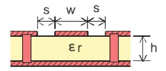
Figure 10-4. Coplanar Waveguide (Cross Section)
