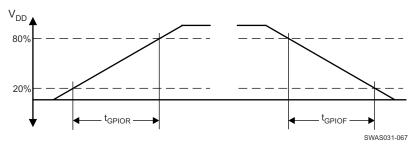
Figure 8-12. GPIO Timing Diagram
