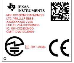
Figure 9-4. CC3220MODAS Module Marking
