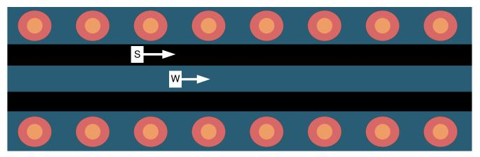
Figure 10-5 shows the top view of the coplanar waveguide with GND and via stitching.
