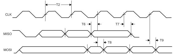
Figure 8-9. SPI Slave Timing Diagram
