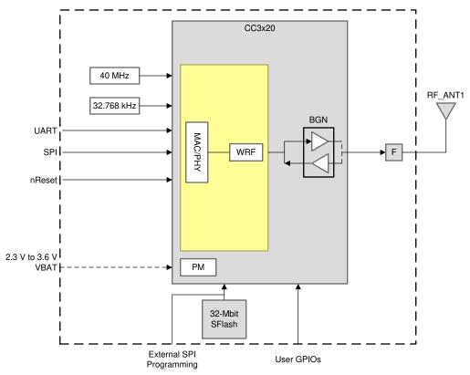
Figure 4-1. CC3220MODx Functional Block Diagram
