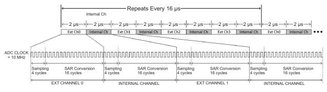
Figure 8-15. ADC Clock Timing Diagram
