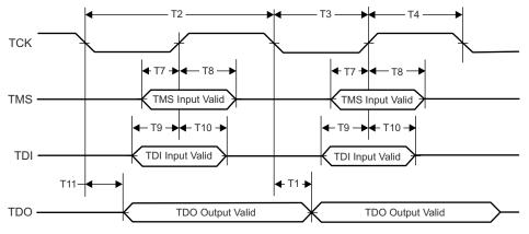
Figure 8-14. JTAG Timing Diagram
