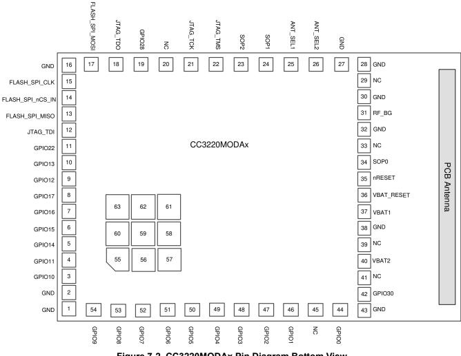
Figure 7-2. CC3220MODAx Pin Diagram Bottom View
