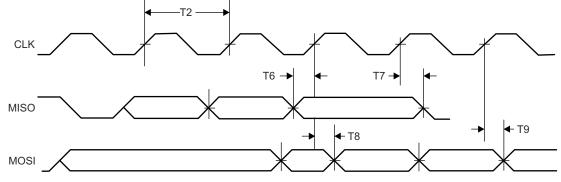
Figure 8-8. SPI Master Timing Diagram
