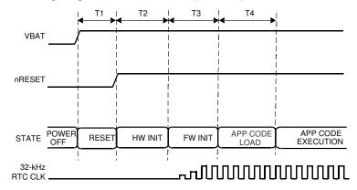
Figure 8-6. First-Time Power-Up and Reset Removal Timing Diagram
