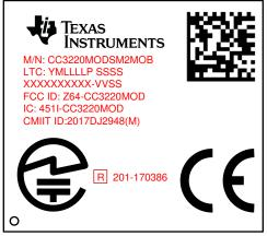
Figure 9-2. CC3220MODS Module Marking
