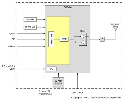
Figure 4-2. CC3220MODAx Functional Block Diagram
