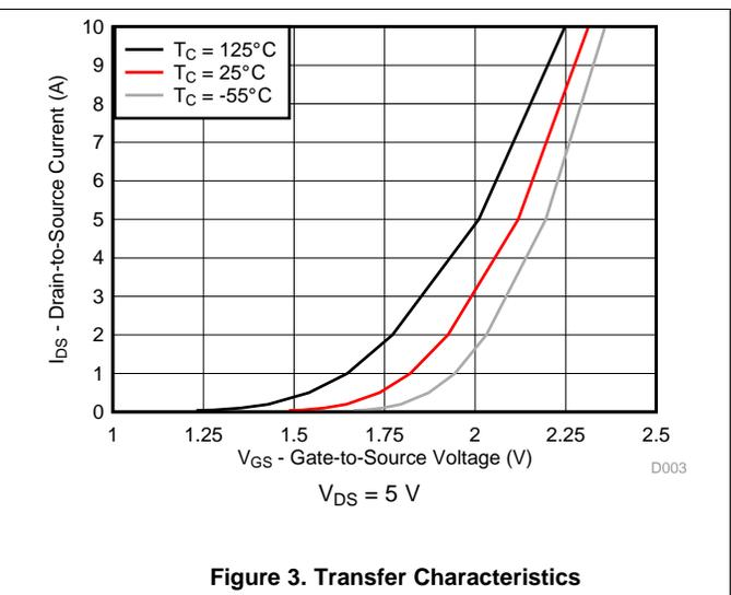
Figure 3. Transfer Characteristics
