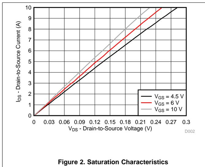
Figure 2. Saturation Characteristics
