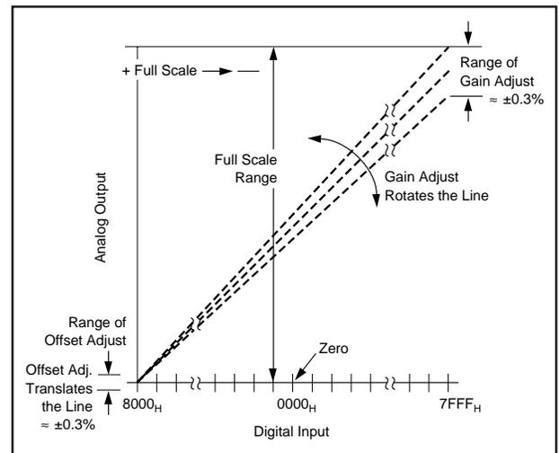
FIGURE 3. Relationship of Offset and Gain Adjustments.
