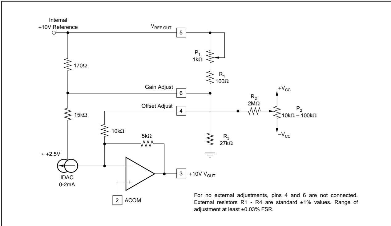
FIGURE 6. Manual Offset and Gain Adjust Circuits.
