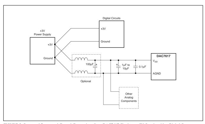
FIGURE 3. Suggested Power and Ground Connections for a DAC7617 Sharing a +3V Supply with a Digital System.
