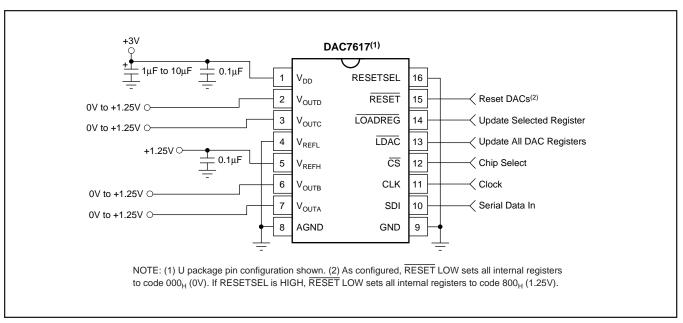
FIGURE 1. Basic Single-Supply Operation of the DAC7617.
