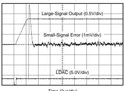
OUTPUT VOLTAGE vs SETTLING TIME (+1.25V to 0V)
