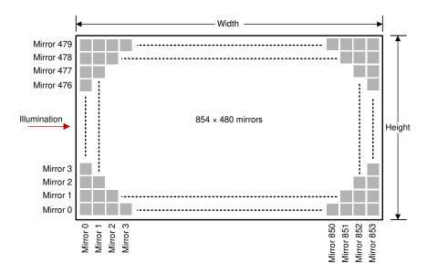
Figure 6-15. Micromirror Array Physical Characteristics
