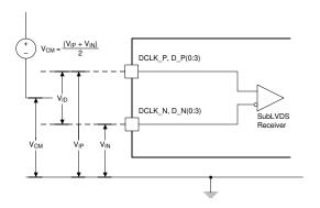
Figure 6-8. SubLVDS Voltage Parameters
