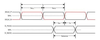
Figure 6-6. SubLVDS Switching Parameters
