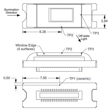
Figure 7-1. DMD Thermal Test Points
