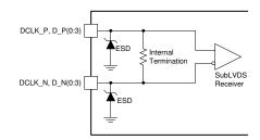
Figure 6-10. SubLVDS Equivalent Input Circuit
