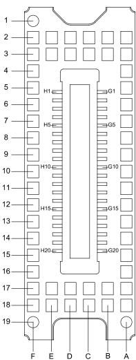
Figure 5-1. FQJ Package 40-Pin Connector Bottom View
