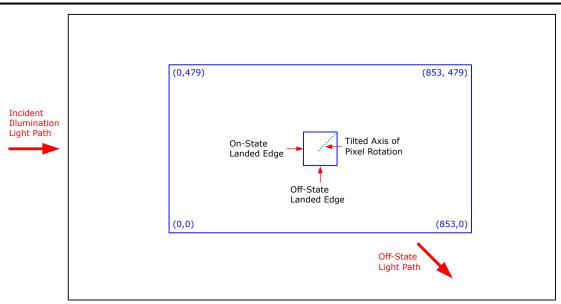
Figure 6-17. Landed Pixel Orientation and Tilt
