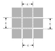
Figure 6-16. Mirror (Pixel) Pitch
