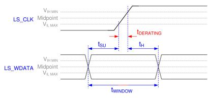
Figure 6-5. Window Time Derating Concept
