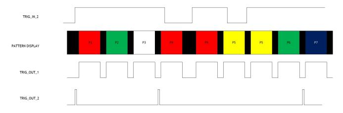
Figure 17. Mode 1 Trigger Timing Diagram
