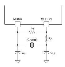
C<sub>L</sub> = crystal load capacitance in F
