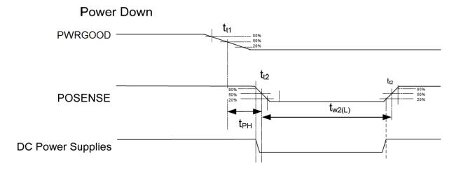
Figure 22. Power-up and Power-down Timing
