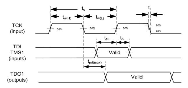
Figure 10. Boundary Scan Timing
