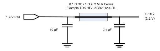
Figure 20. FPD-Link 1.2-V Power Pin Configuration
