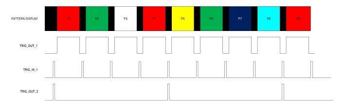
Figure 16. Mode 1 Triggers Timing Diagram for 6-bit Patterns
