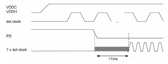
Figure 2. LVDS Timing Diagram
