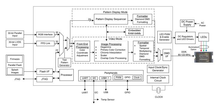
Figure 13. DLPC350 Functional Block Diagram
