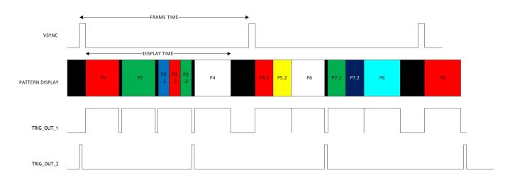
Figure 15. Mode 0 Trigger Timing Diagram
