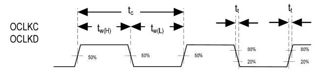
Figure 8. Programmable Output Clocks Timing Diagram
