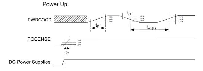
PWRGOOD has no impact on operation for 60 ms after rising edge of POSENSE.
