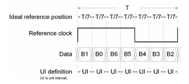
Figure 3. (LVDS) Link Start-up Timing
