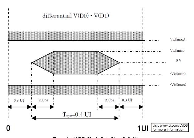
Figure 4. (LVDS) Clock: Data Skew Definition
