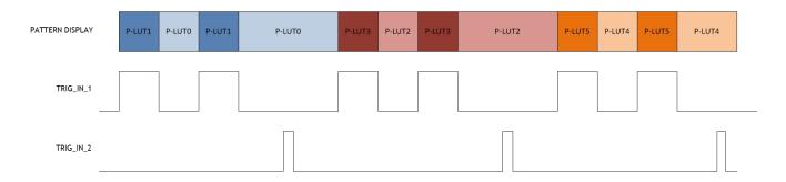
Figure 18. Mode 2 Trigger Timing Diagram
