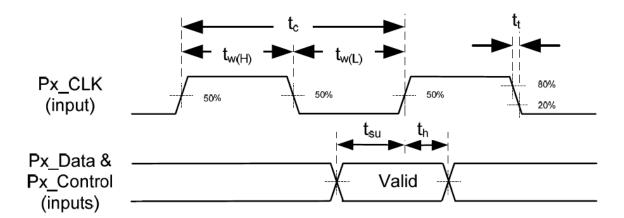
Figure 1. Port 1 Input Pixel Timing
