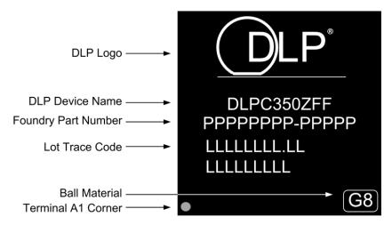
Figure 29. Device Marking
