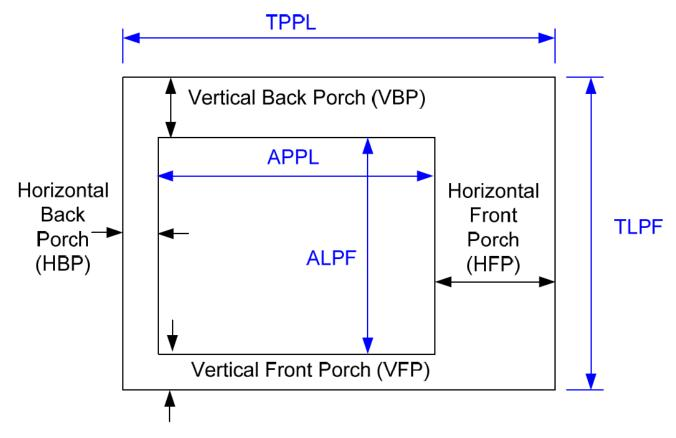
Figure 6. Horizontal and Vertical Blanking Diagram
