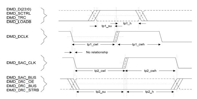
Figure 9. DMD Interface Timing
