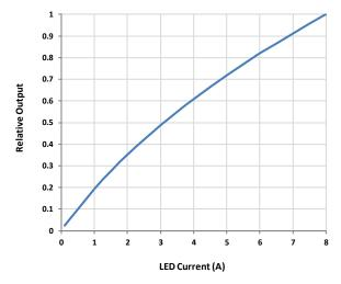
Figure 15. Relative Output vs LED Current
