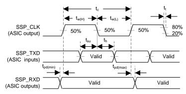
Figure 10. Synchronous Serial Port Interface
