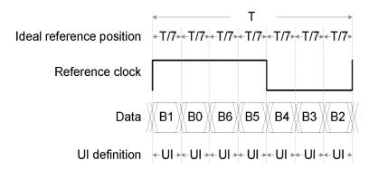
Figure 9. (LVDS) Clock - Data Skew Definition
