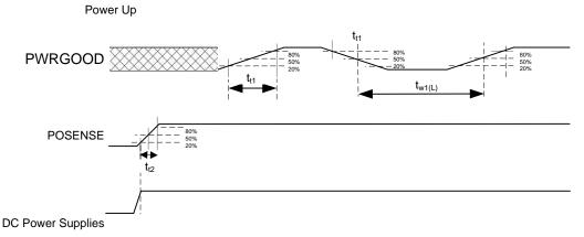
PWRGOOD has no impact on operation for 60 ms after rising edge of POSENSE.
