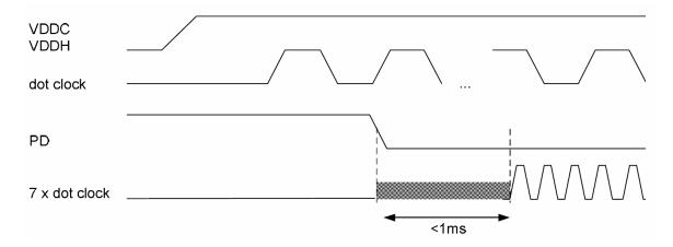
Figure 8. (LVDS) Link Start-Up Timing
