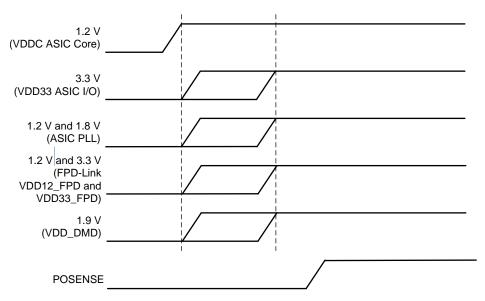
Figure 16. System Power-Up Sequence
