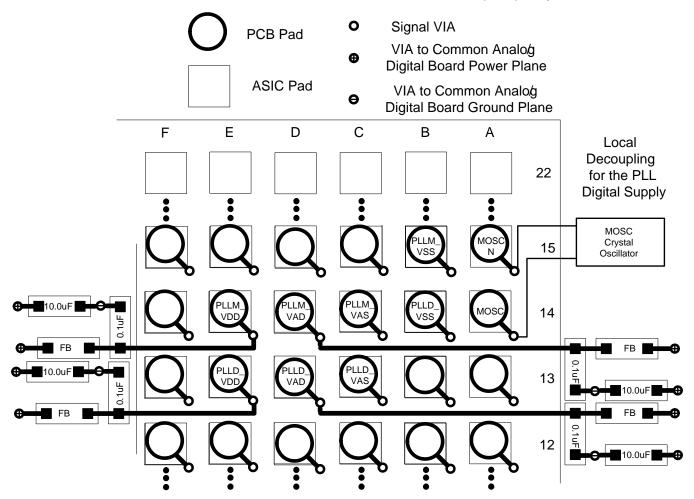
Figure 18. PLL Filter Layout
