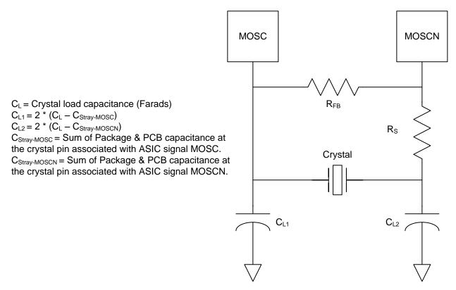
Figure 14. Recommended Crystal Oscillator Configuration
