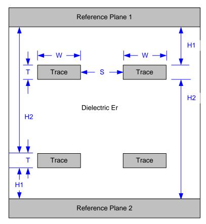
Figure 19. PCB Stackup Geometries
