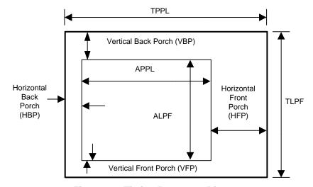
Figure 22. Timing Parameter Diagram
