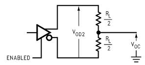
Figure 1. Driver  $V_{OD}$  and  $V_{OC}^{(1)}$
