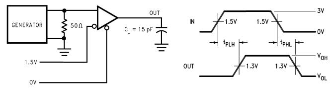
Figure 7. Receiver Propagation Delay Times (5)(6)
