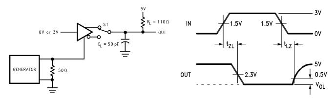
Figure 6. Driver Enable and Disable Times ( $t_{ZL}$ ,  $t_{LZ}$ )  $^{(5)(6)(7)}$
