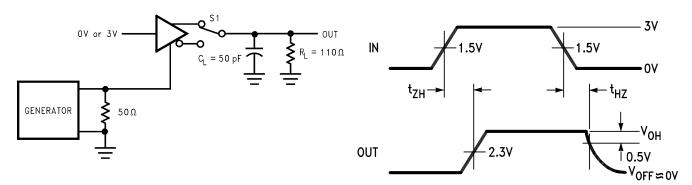
Figure 5. Driver Enable and Disable Times  $(t_{ZH}, t_{HZ})^{(2)(4)(3)}$
