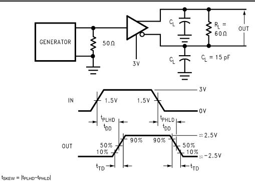
Figure 3. Driver Differential Output Delay and Transition Times $^{(2)(3)}$
