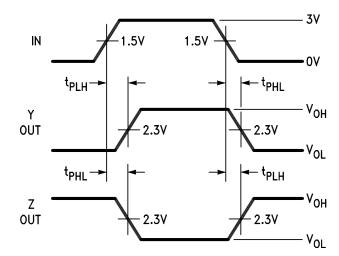
Figure 4. Driver Propagation Times (2)(4)
