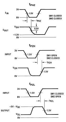
Figure 3. Propagation Delay TRI-STATE Control Input to Output
