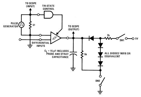
1.5V for  $t_{PHZ}$  and  $t_{PLZ}$ 1.5V for  $t_{PLZ}$  and  $t_{PZL}$ Input pulse characteristics:  $t_{TLH} = t_{THL} = 6$  ns (10% to 90%) PRR = 1 MHz, 50% duty cycle
