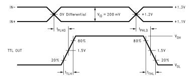
Figure 5-2. Receiver Propagation Delay and Transition Time Waveforms
