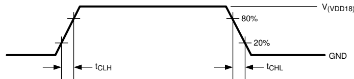
Figure 6-1. LVCMOS Transition Times
