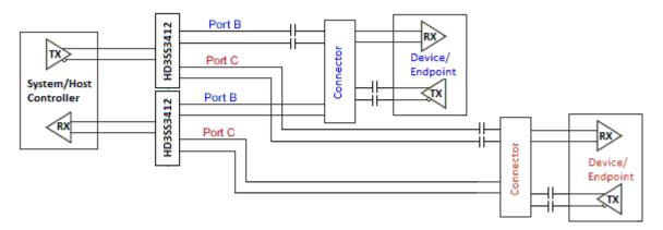
Figure 11. AC Coupling Capacitors Between Switch Tx and Endpoint Tx
