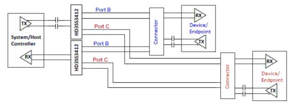
Figure 12. AC Coupling Capacitors on Host Tx and Endpoint Tx
