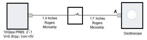
Figure 10. Output Eye Diagram Test Setup
