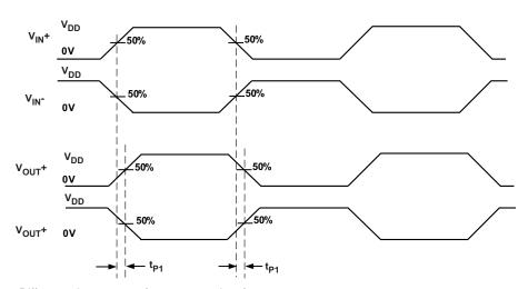
$T_{SKEWInter}$  = Difference between  $t_{PD}$  for any two pairs of outputs
