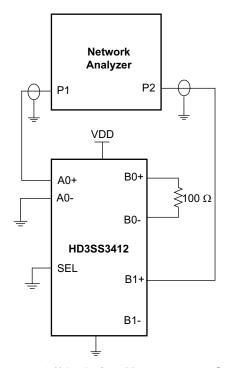
Figure 8. Off Isolation Measurement Setup
