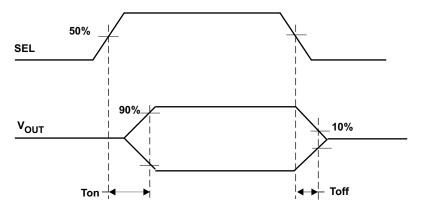
Figure 1. Switch ON and OFF Timing Diagram
