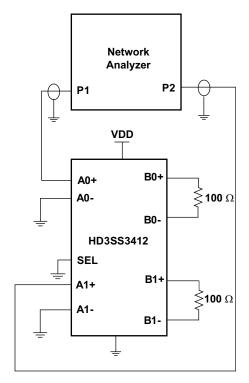
Figure 7. Cross Talk Measurement Setup
