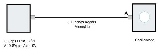
Figure 9. Source Eye Diagram Test Setup
