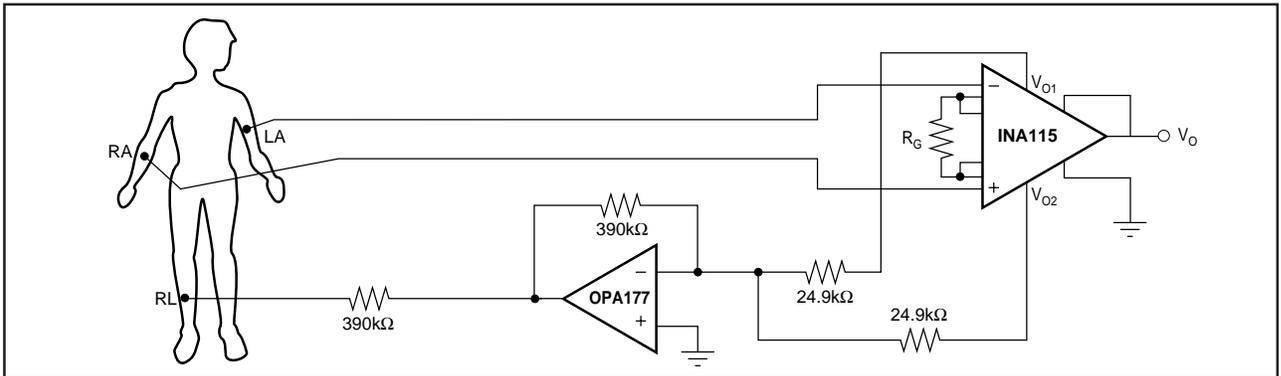
FIGURE 7. ECG Amplifier with Right Leg Drive.
