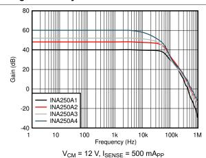
Figure 6-16. Amplifier Gain vs Frequency
