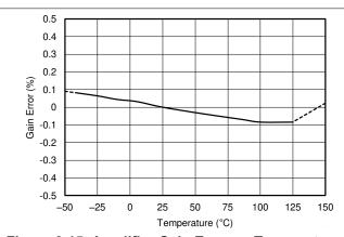
Figure 6-15. Amplifier Gain Error vs Temperature
