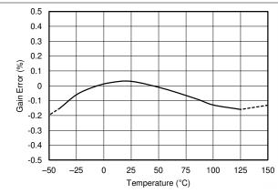
Figure 6-13. System Gain Error vs Temperature
