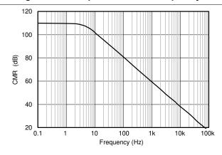
VS = 5 V,  $V_{REF} = 2.5 \text{ V}$ ,  $I_{SENSE} = 0 \text{ A}$ ,  $V_{CM} = 1 \text{-V}$  sine wave
