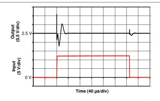
Input = VIN+,  $V_{REF}$  = 2.5 V
