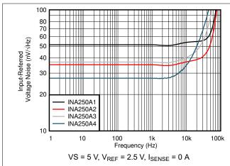
Figure 6-25. Input-Referred Voltage Noise vs Frequency
