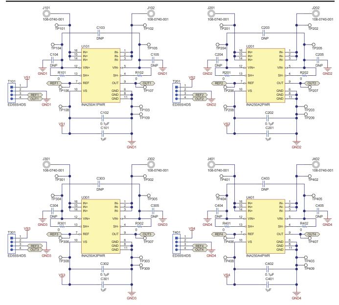
Figure 8-8. Recommended Layout Schematic
