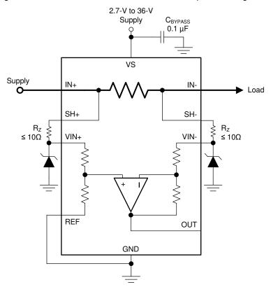
Figure 7-7. Device Transient Protection
