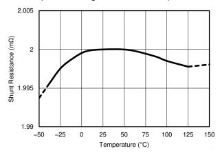
Figure 7-3. Sensing Resistor vs Temperature
