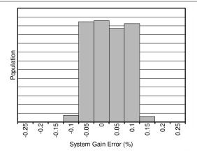
System gain error = R<sub>SHUNT</sub> error + amplifier gain error, load current = 10 A
