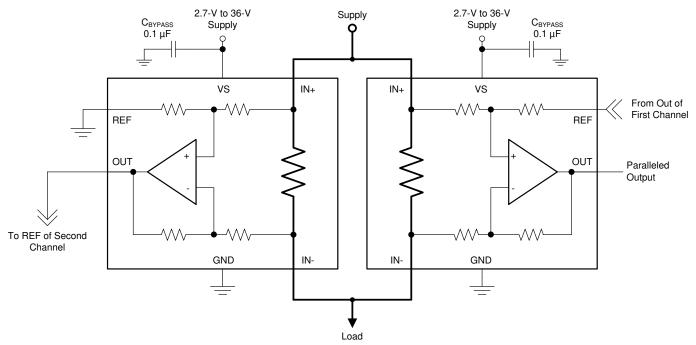
Figure 8-3. Parallel Summing Configuration
