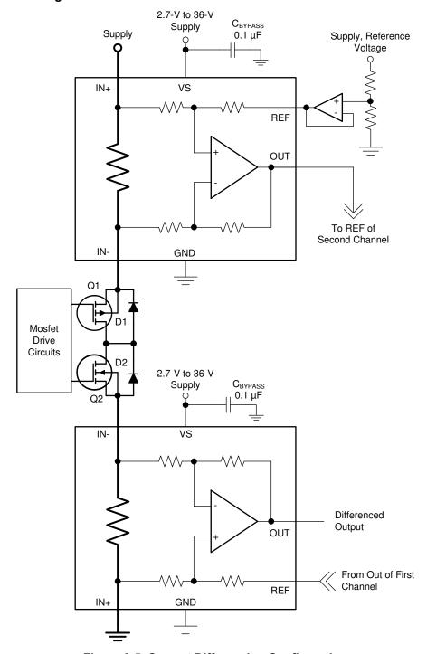
Figure 8-5. Current Differencing Configuration
