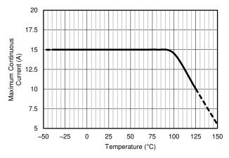
Figure 7-1. Maximum Current vs Temperature
