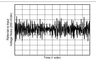
VS = 5 V,  $V_{CM} = 0 V$ ,  $I_{SENSE} = 0 A$
