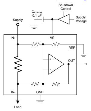
Figure 7-6. Shutting Down the Device
