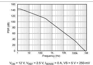
Figure 6-17. Power-Supply Rejection vs Frequency
